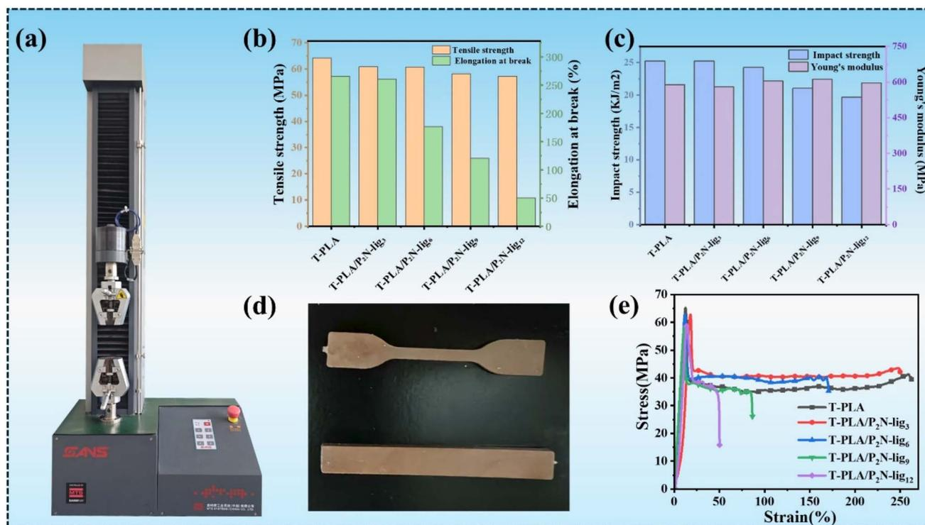
Fig. 6 Mechanical properties of T-PLA/P<sub>2</sub>N-lig: (a) optical images of the CMT2503 equipment, (b) tensile testing, (c) impact testing and Young's modulus, (d) test spline optical photographs, (d) stress–strain curves.
