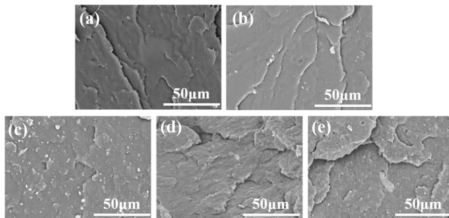
Fig. 7 SEM images of the fracture surfaces after impact testing of T-PLA/P<sub>2</sub>N-lig: (a) T-PLA, (b) T-PLA/P<sub>2</sub>N-lig<sub>3</sub>, (c) T-PLA/P<sub>2</sub>N-lig<sub>6</sub>, (d) T-PLA/P<sub>2</sub>N-lig<sub>9</sub>, (e) T-PLA/P<sub>2</sub>N-lig<sub>12</sub>.
