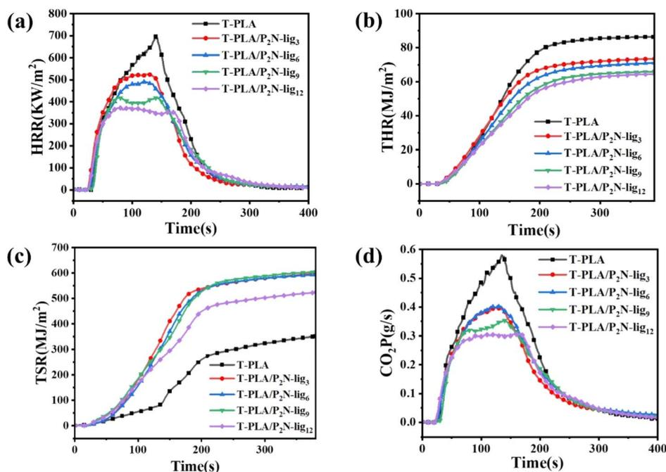
Fig. 4 Cone calorimetry profiles of T-PLA/P<sub>2</sub>N-lig: (a) HRR, (b) THR, (c) TSR, (d) CO<sub>2</sub>P.
