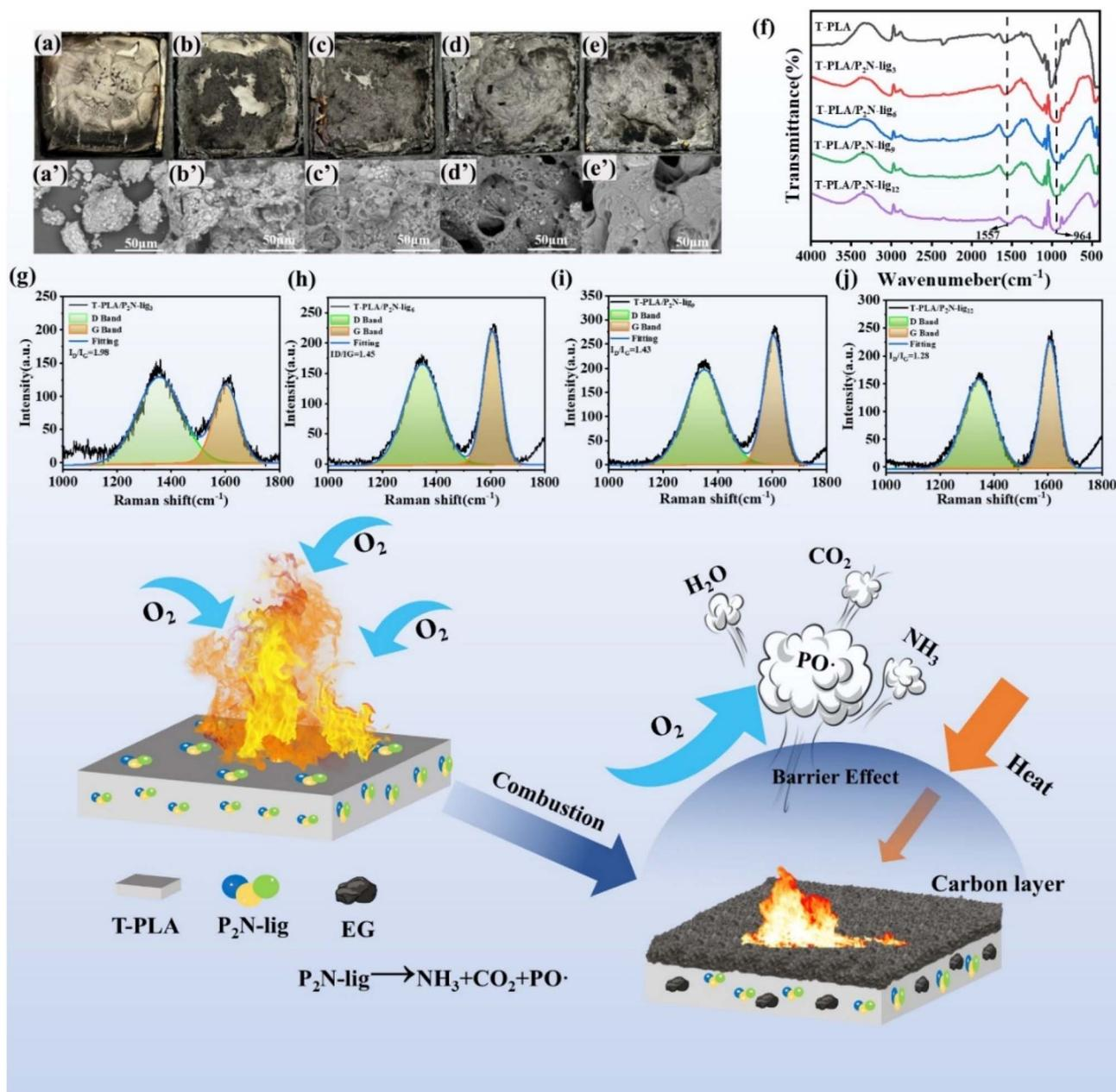
Fig. 5 Char residue analysis of T-PLA/P<sub>2</sub>N-lig FR composites.
