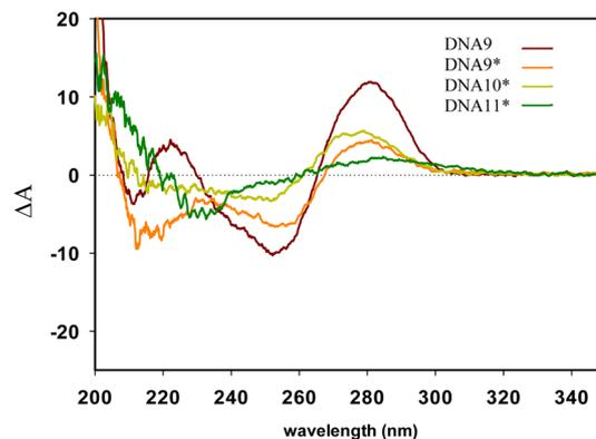
Fig. 4 Comparison of CD spectra at 5 °C of non-modified DNA9 and corresponding modified sequences of DNA9<sup>A\*</sup>, DNA10<sup>A\*</sup> and hyper-modified DNA11<sup>A\*</sup>.
