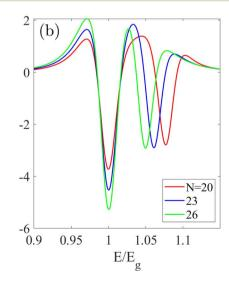
Fig. 4 The quadratic electro-optic (DC Kerr) effect for (a)  $S_1$  and (b)  $S_2$  BPNTs. The spectra show that as the nanotube radius increases, peak intensities grow for energies below the band gap, while peaks at  $E > E_q$  exhibit a noticeable red-shift.
