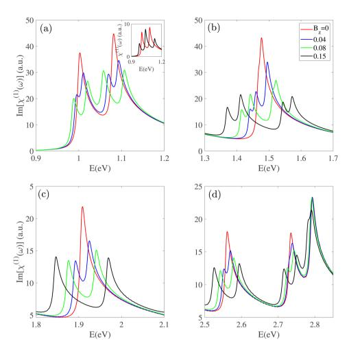
Fig. 7 (a)–(d) The effect of an axial magnetic field (Bz) on the linear susceptibility of a Z20-BPNT. The application of a magnetic field lifts subband degeneracy, leading to the splitting of each original optical peak into two components, one red-shifted and one blue-shifted.
