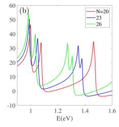
Fig. 2 The real part of the linear optical susceptibility for (a)  $S_1$  and (b)  $S_2$  nanotube types. The static dielectric constant ( $\omega \to 0$ ) is shown to increase with the nanotube radius and the spectral peaks undergo the radius-dependent red-shifts.
