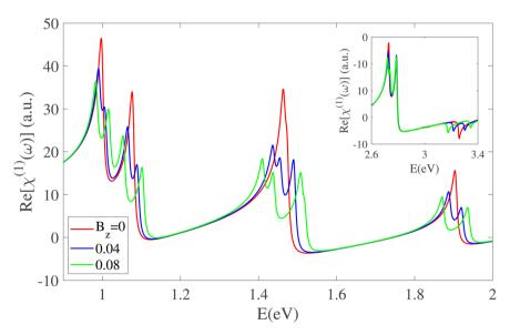
Fig. 8 The real part of the linear susceptibility under an axial magnetic field. The results highlight pronounced splitting of peaks across both the infrared and visible ranges.
