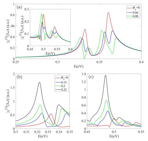
Fig. 11 (a–c) The third-harmonic generation spectrum under an increasing magnetic field in the different energy regions. THG peaks located near  $E_g/3$  and  $E_g/2$  progressively split into multiple components as  $B_z$  increases, while stronger fields lead to a pronounced enhancement of their intensities.
