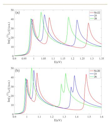
Fig. 1 The imaginary part of the linear optical susceptibility for two families of zigzag BPNTs (a)  $S_1$  and (b)  $S_2$ . The spectra show a systematic red-shift of the primary infrared absorption peaks as the nanotube radius increases.
