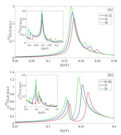
Fig. 6 The third-harmonic generation spectrum for (a)  $S_1$  and (b)  $S_2$  nanotube types. The dominant THG peak occurs at approximately  $E_g/3$ , with its intensity increasing and exhibiting a red-shift as the nanotube radius grows. Unlike CNTs, BPNTs show multi-peak THG features, highlighting their unique nonlinear response arising from their intrinsic semiconducting character.
