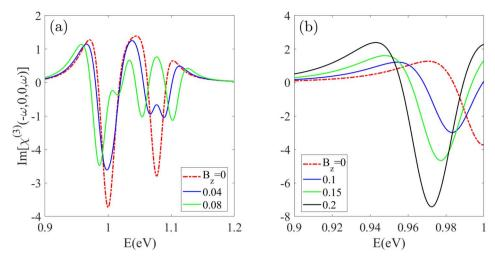
Fig. 9 The DC Kerr effect spectrum for a Z20-BPNT under (a) weak and (b) strong magnetic fields. The applied field induces peak splitting, redshifts, and intensity modifications across the infrared range.
