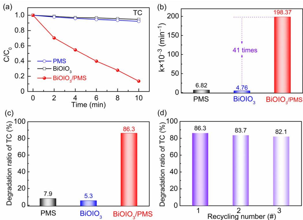
Fig. 4 (a) Catalytic degradation curves ( $C/C_0$  vs. time) of various systems towards TC solution. (b) Reaction kinetic constants of PMS,  $\text{BiOI}_3$  and  $\text{BiOI}_3/\text{PMS}$  for TC solution. (c) Degradation ratio of PMS,  $\text{BiOI}_3$  and  $\text{BiOI}_3/\text{PMS}$ . (d) Degradation ratio of  $\text{BiOI}_3/\text{PMS}$  after the recycling tests.
