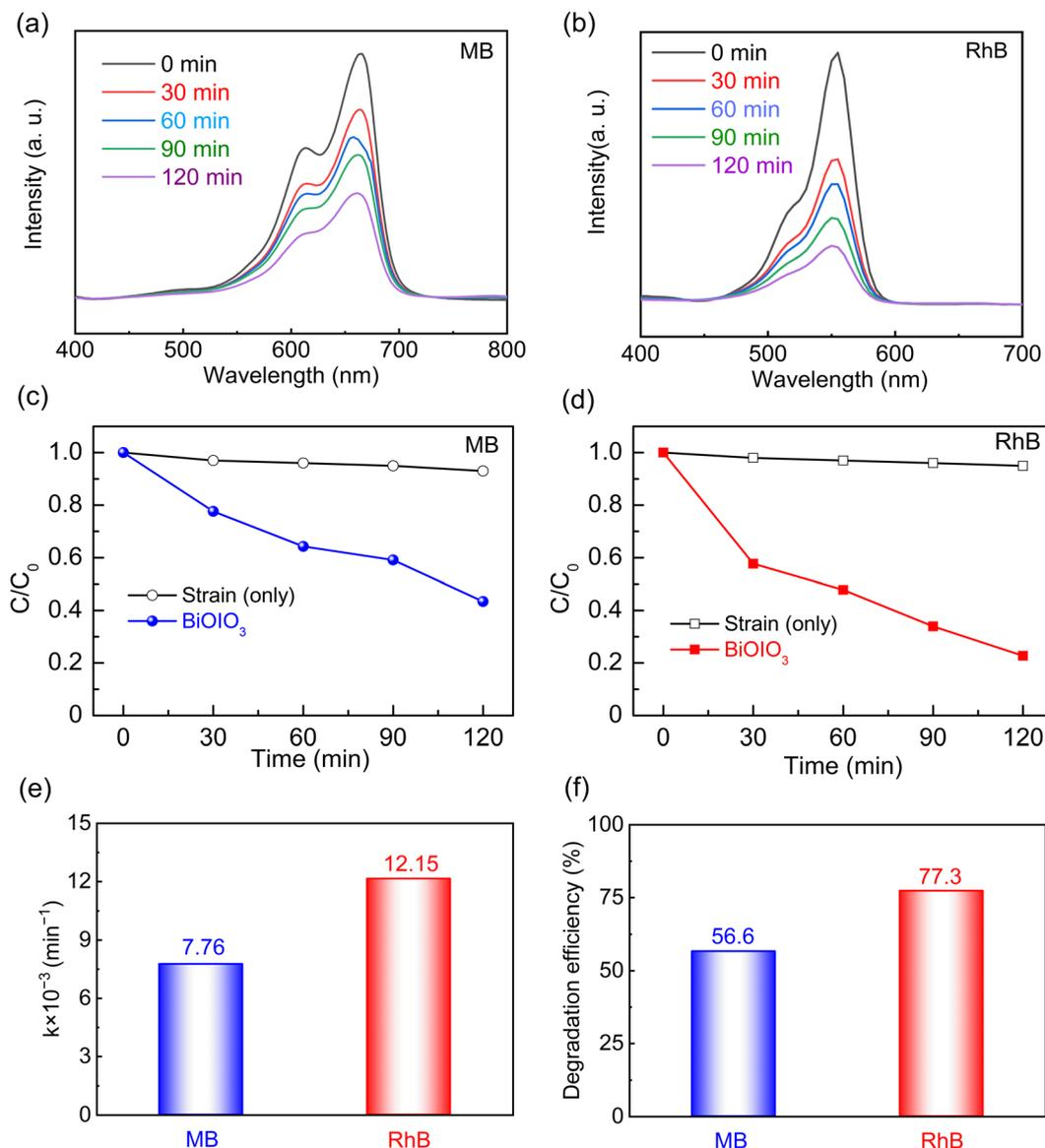
Fig. 2 UV-vis absorption spectra of piezocatalytic degradation for (a) MB and (b) RhB solutions at different time intervals with BiOIO<sub>3</sub>. Piezocatalytic degradation curves ( $C/C_0$  vs. time) of the strain (only) and BiOIO<sub>3</sub> towards (c) MB and (d) RhB solutions. (e) Piezocatalytic degradation kinetic constants and (f) corresponding degradation efficiency of BiOIO<sub>3</sub> towards MB and RhB solutions.
