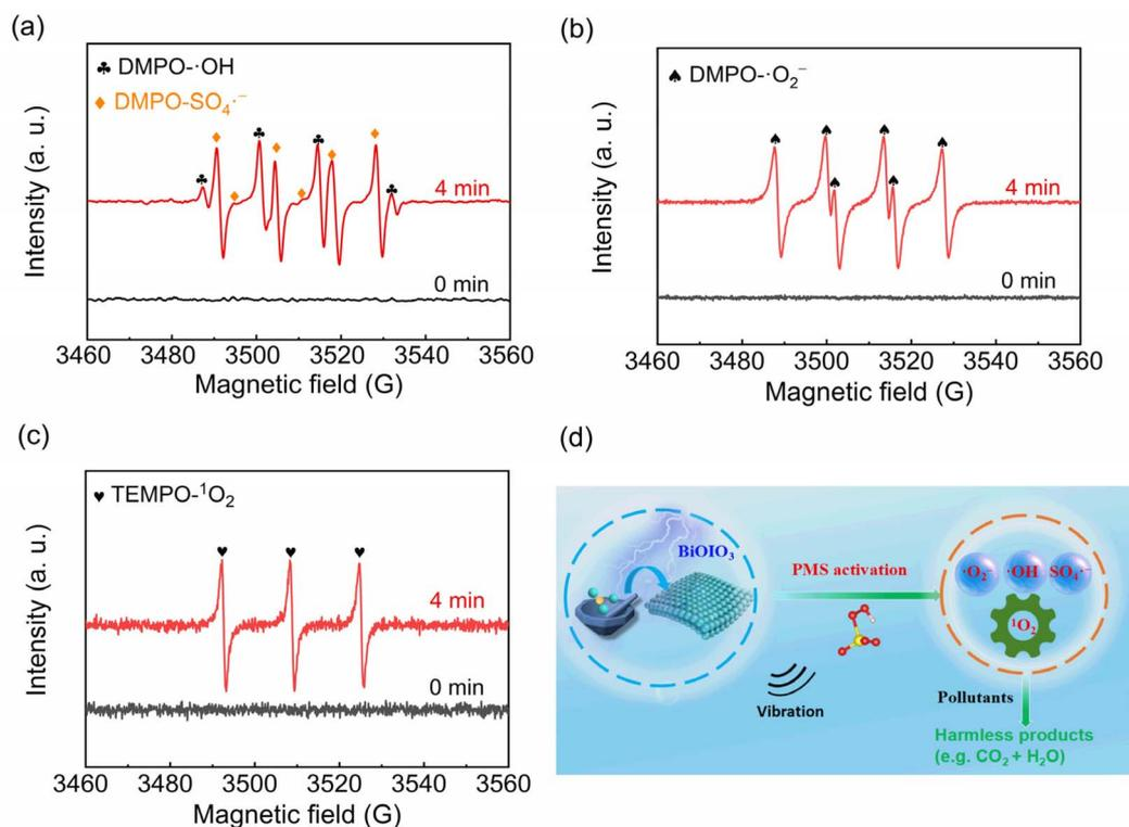
Fig. 6 EPR detection for (a)  $\cdot\text{OH}/\text{SO}_4\cdot^-$ , (b)  $\cdot\text{O}_2^-$  and (c)  $^1\text{O}_2$  in  $\text{BiOI}/\text{O}_3/\text{PMS}$  under various ultrasonic vibration conditions. (d) Mechanism of the piezocatalytic activation of PMS for the degradation of pollutants over  $\text{BiOI}/\text{O}_3$ .
