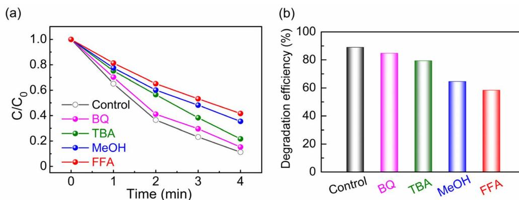
Fig. 5 (a)  $C/C_0$ -time plots and (b) degradation efficiency of RhB dye over BiOIO<sub>3</sub>/PMS with the various radical scavengers under ultrasonic vibration.
