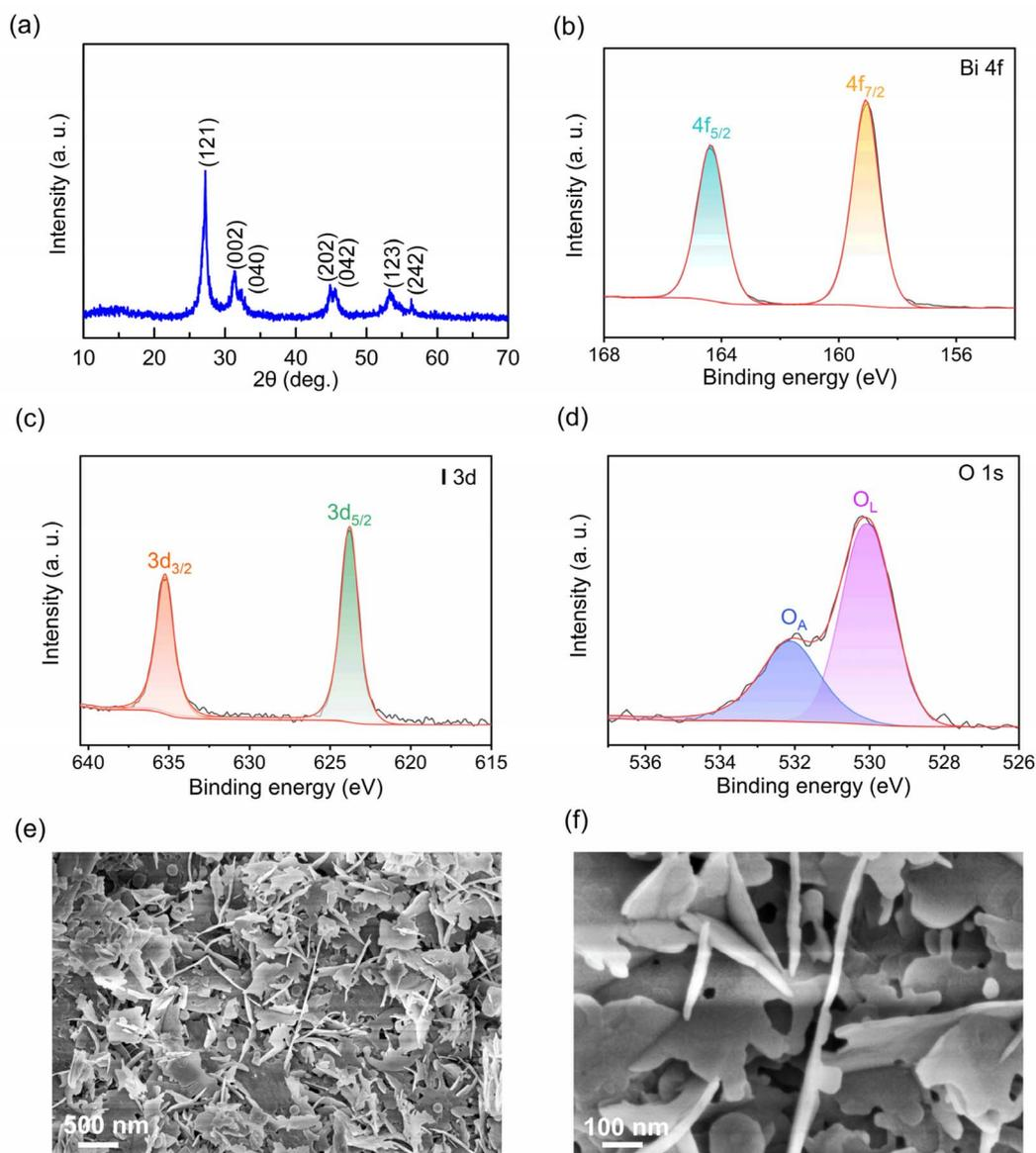
Fig. 1 (a) XRD pattern of BiIO<sub>3</sub>. High-resolution XPS spectra of (b) Bi 4f, (c) I 3d, and (d) O 1s for BiIO<sub>3</sub>. (e–f) SEM images of BiIO<sub>3</sub>.
