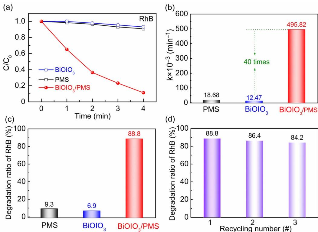
Fig. 3 (a) Catalytic degradation curves ( $C/C_0$  vs. time) of various systems towards RhB solution. (b) Reaction kinetic constants of PMS,  $\text{BiOI}_3$  and  $\text{BiOI}_3/\text{PMS}$  for the degradation of RhB solution. (c) Degradation ratio of PMS,  $\text{BiOI}_3$  and  $\text{BiOI}_3/\text{PMS}$ . (d) Decomposition ratio of  $\text{BiOI}_3/\text{PMS}$  after the recycling tests.
