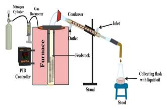
Fig. 1 Schematic representation of experimental setup
