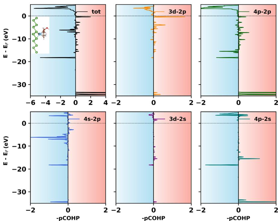
Fig. 12 Total and orbital-wise partial crystal orbital Hamiltonian population ( $-\text{pCOHP}$ ) for Ti–C bonding pair in  $\text{As}_{50}\text{Ti}$ /molecule. Positive (negative) values of  $-\text{pCOHP}$  correspond to bonding (antibonding) states. The Fermi level is at 0 eV, marked in a dotted line. For better comparison, the x-axis scale is set the same for all orbital interactions.
