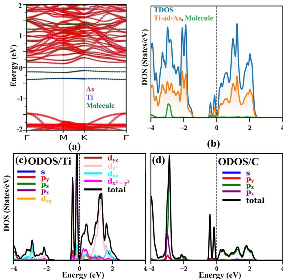
Fig. 9  $\text{As}_{50}\text{Ti}$  with molecule in the lowest energy configuration; (a) band structure, (b) total density of states, (c) orbital density of states (ODOS) for Ti-atom, and (d) ODOS for C-atom.
