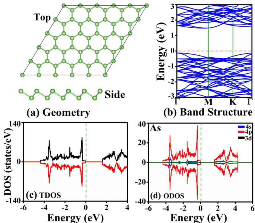
Fig. 1 Pristine arsenene; (a) relax geometry, (b) band structure, (c) total density of states (TDOS), (d) orbital DOS (ODOS). The Fermi level ( $E_F$ ) is set at 0 eV.
