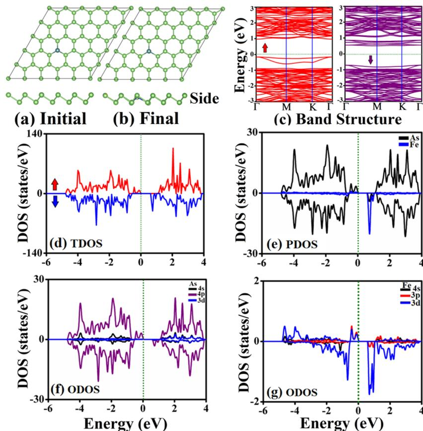
Fig. 2 Single Fe-atom doped arsenene ( $\text{As}_{49}\text{Fe}$ ): (a) initial structure, (b) final structure, (c) band structure, (d) TDOS, (e) PDOS of As and Fe-atom, (f) ODOS of As-atom, (g) ODOS of Fe-atom.
