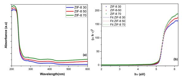
(a) Absorption spectrum, (b) and Tauc's spectrum of ZIF-8 powders.
