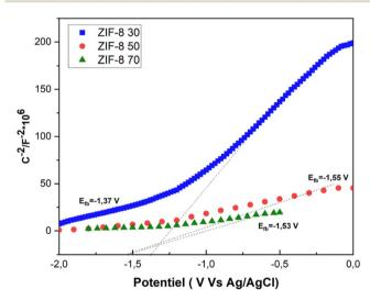
Fig. 14 M-S plots of ZIF-8 30, ZIF-8 50 and ZIF-8 70
