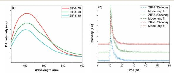
Fig. 15 (a) PL spectrum of ZIF-8 catalysts. (b) TRFL (lifetime-decay) plot of the ZIF-8 materials.
