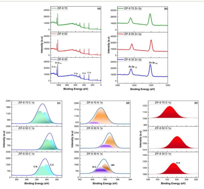
Fig. 5 (a) XPS wide scan of the prepared ZIFs (ZIF-8 70, ZIF-8 50, ZIF-8 30); (b) Zn 2p spectra; (c) C 1s Spectra; (d) N 1s Spectra and (e) O 1s spectra off the prepared ZIFs.
