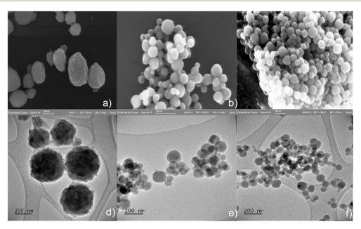
Fig. 3 SEM and TEM images of ZIF-8 samples: (a and d) ZIF-8.30 (b and e) ZIF-8.50 and (c and f) ZIF-8.70.
