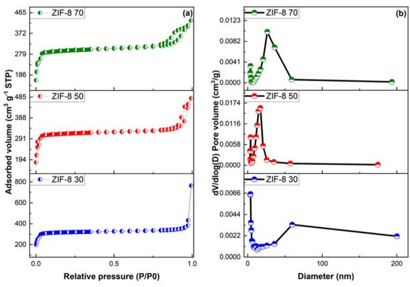
Fig. 4 (a) N<sub>2</sub> adsorption/desorption isotherms of ZIF-8 synthesized materials and (b) pore distribution of ZIF-8 materials using BJH method.
