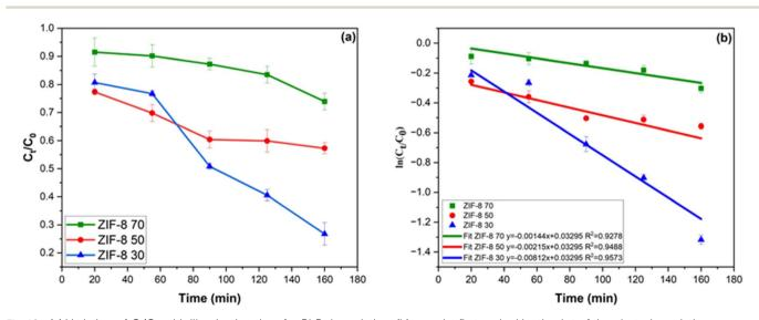
Fig. 12 (a) Variation of  $C_t/C_0$  with illumination time for RhB degradation, (b) pseudo-first-order kinetic plot of the photodegradation process.
