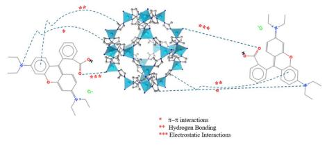
Suggested mechanism of rhodamine B adsorption onto ZIF-8.70
