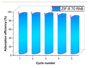
Fig. 11 Effect of recovery cycles on the removal efficiency of Rh-B onto ZIF-8.70
