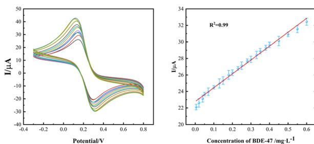
Fig. 8 Linear equation of BDE-47 (vs. Ag/AgCl reference electrode).
