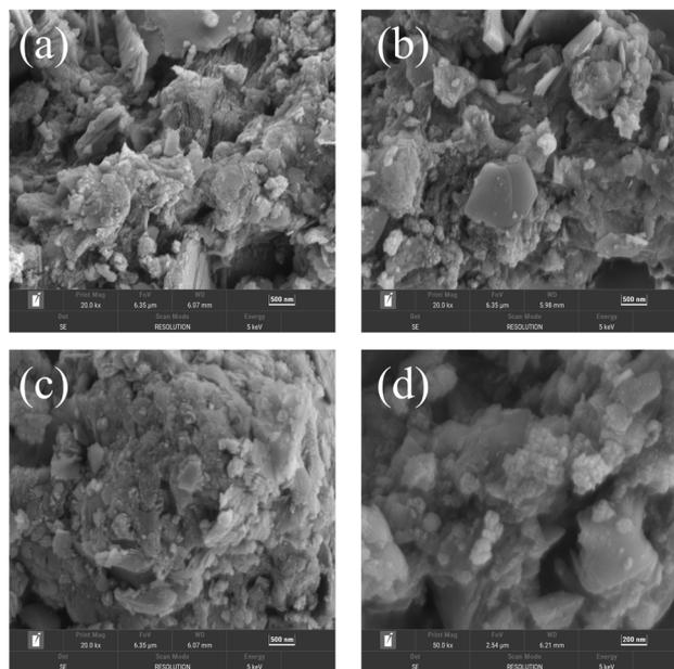
Fig. 3  $20\times$  FESEM images of sludge biochar produced by pyrolysis at  $400^\circ \text{C}$ ,  $600^\circ \text{C}$ , and  $800^\circ \text{C}$  (a–c) and  $50\times$  image of biochar pyrolyzed at  $600^\circ \text{C}$  (d).
