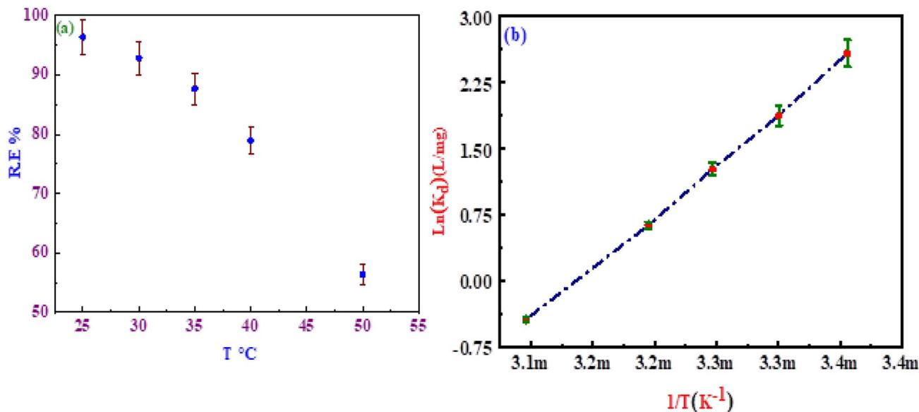
Fig. 6 (a) Effect of temperature on CFX removal efficiency at pH 8 using the LDH/CA nanocomposite and (b) for the thermodynamic parameters can be estimated by examining  $\ln K_d$  changes with temperature ( $K$ ).
