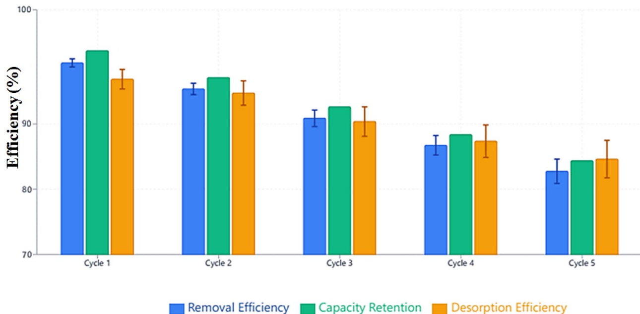
Fig. 11 Reusability of Zn-Fe LDH/CA composite for CFX removal over five consecutive adsorption-desorption cycles.
