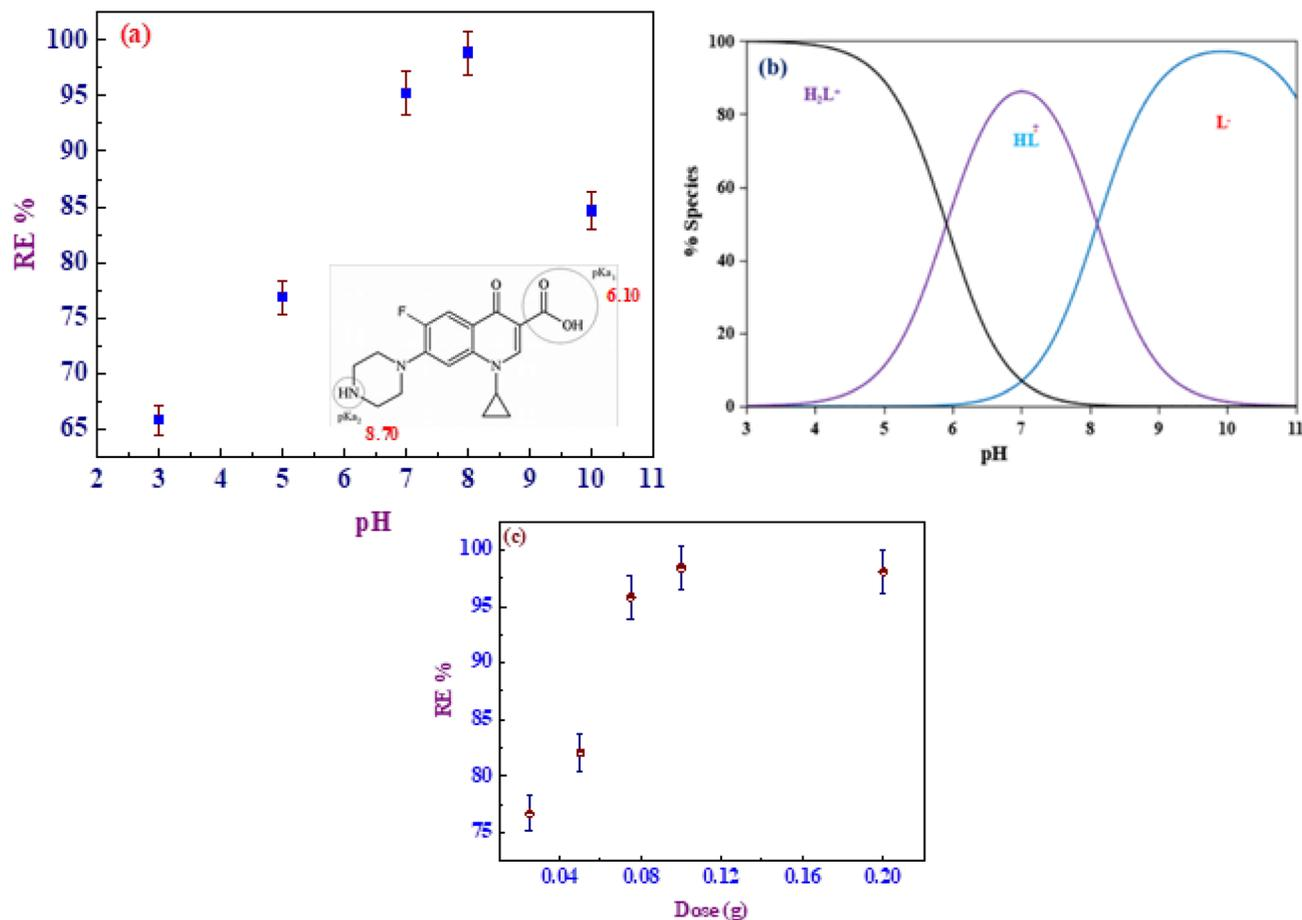
Fig. 5 (a) Adsorption of CFX at different pH values for the 50  $\mu\text{g mL}^{-1}$  solution of CFX by Zn–Fe LDH/CA (0.075 g/50 mL) at 25  $^{\circ}\text{C}$ ; the inset structure of CFX; (b) species distribution curve of CFX at different pH values; and (c) effect of adsorbent dose on CFX adsorption at a concentration of 50  $\mu\text{g mL}^{-1}$  and a volume of 50 mL at pH 8.
