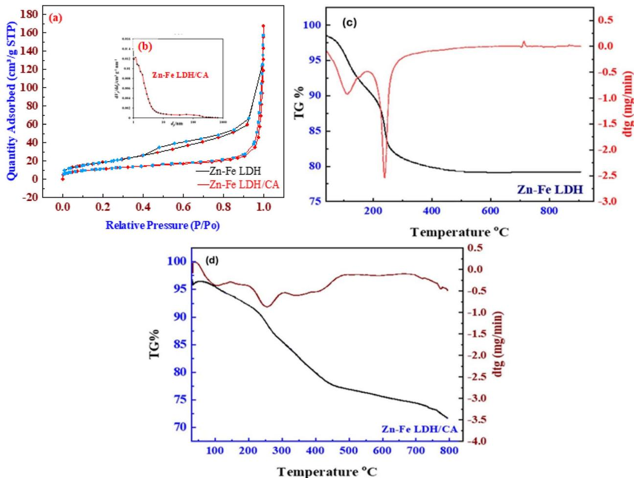
Fig. 4 (a) Adsorption–desorption isotherms of  $N_2$ ; (b) pore diameter distribution curves for the various samples under study and TGA/DTG thermograms of (c) Zn–Fe LDH and (d) Zn–Fe LDH/CA.
