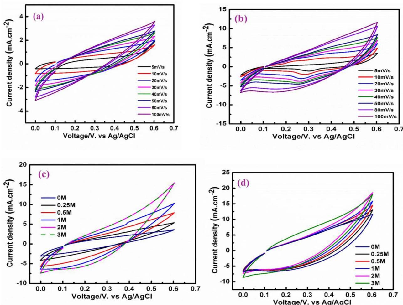
Fig. 9 Effect of scan rate on (a) CV curves of Zn-Fe LDH/CA before, (b) Zn-Fe LDH/CA after adsorption and effect of methanol concentration on (c) CV of Zn-Fe LDH/CA before and (d) Zn-Fe LDH/CA after adsorption.
