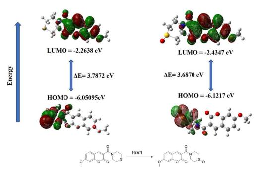
Fig. 4 HOMO-LUMO energy gap of probe W-HOCl before and after addition of HOCl.
