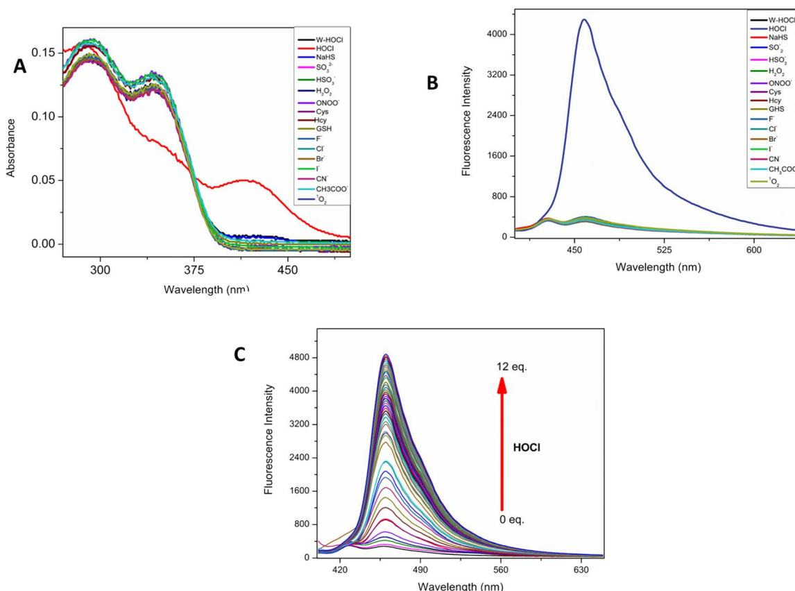
Fig. 1 (A) The electronic absorption spectra of probe W-HOCl (10 μM) (B) F<sub>1</sub> selectivity of probe (C) F<sub>1</sub> titration of probe with HOCl (10 eq.) in HEPES buffer (10 mM, pH = 7.4, having 60% EtOH).
