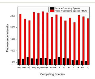
Fig. 2 FL response of W-HOCl (10  $\mu$ M) with HOCl (10 eq.) at 460 nm changes upon addition of ions in the presence of HOCl (10 eq.) in HEPES buffer (10 mM, pH = 7.4, having 60% EtOH,  $\lambda_{ex}$  = 380 nm, slit: 5 nm)
