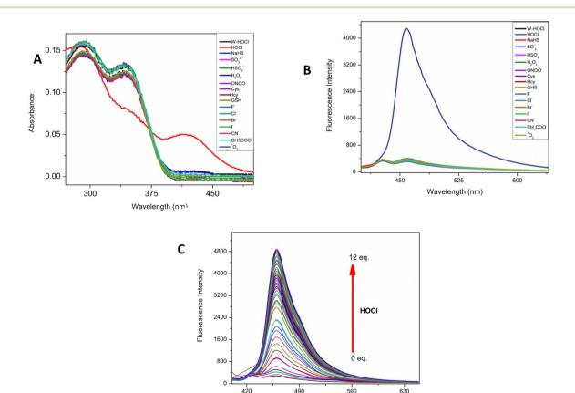
Fig. 1 (A) The electronic absorption spectra of probe W-HOCl (10  $\mu$ M) (B)  $F_l$  selectivity of probe (C)  $F_l$  titration of probe with HOCl (10 eq.) in HEPES buffer (10 mM, pH = 7.4, having 60% EtOH).
