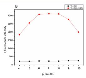
Fig. 3 FL response of W-HOCl (10  $\mu$ M) at 460 nm when treated with HOCl ions (10 eq.) (A) with time (B) at different pH in HEPES buffer (10 mM, pH = 7.4, having 60% EtOH,  $\lambda_{ex}$  = 380 nm, slit: 5 nm).
