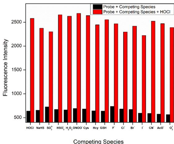
Fig. 2 FL response of W-HOCl (10 μM) with HOCl (10 eq.) at 460 nm changes upon addition of ions in the presence of HOCl (10 eq.) in HEPES buffer (10 mM, pH = 7.4, having 60% EtOH, λ<sub>ex</sub> = 380 nm, slit: 5 nm).
