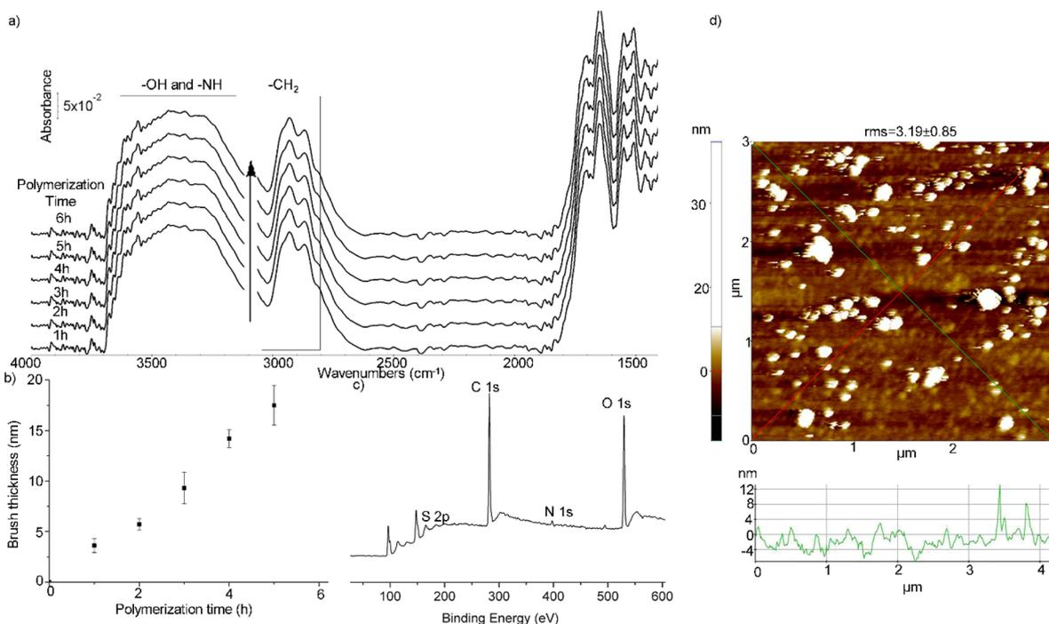
**Fig. 7** (a) ATR-FTIR spectra of the P2 brush surface obtained after different polymerization times (1 h to 6 h), labelled on each spectrum. (b) Variation of brush thickness with polymerization time for the P2 brush surface. (c) XPS survey spectrum of the P2 brush surface after 6 hours of polymerization (polymer thickness  $\approx$  17.5 nm). (d) 2D-AFM image of the P2 brush surface after 6 hours of polymerization (polymer thickness  $\approx$  17.5 nm).
