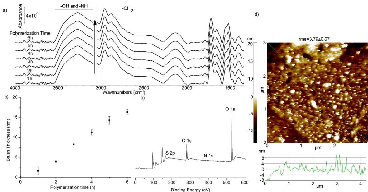
**Fig. 6** (a) ATR-FTIR spectra of the P1 brush surface obtained after different polymerization times (1 h to 6 h), labelled on each spectrum. (b) Variation of brush thickness with polymerization time for the P1 brush surface. (c) XPS survey spectrum of the P1 brush surface after 6 hours of polymerization (polymer thickness  $\approx$  16 nm). (d) 2D-AFM image of the P1 brush surface after 6 hours of polymerization (polymer thickness  $\approx$  16 nm).
