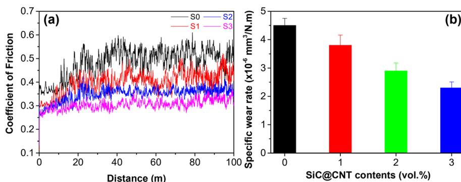
Fig. 7 (a) Friction coefficient and (b) specific wear rate of prepared samples.
