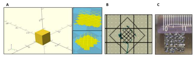
Fig. 9 3D designing (A) CAD models designed, (B) G-CODE generated, and (C) 3D printed with GelMA.
