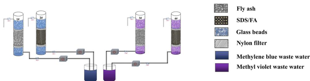
Fig. 1 SDS/FA dynamic test device system.
