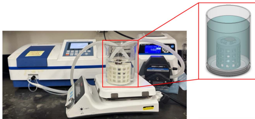
Fig. 1 Image of experimental set up for continuous caffeine release studies using the UV-vis spectrometer and flow-through cuvette.
