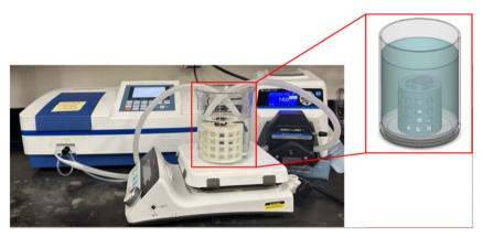
Fig. 1 Image of experimental set up for continuous caffeine release studies using the UV-vis spectrometer and flow-through cuvette.
