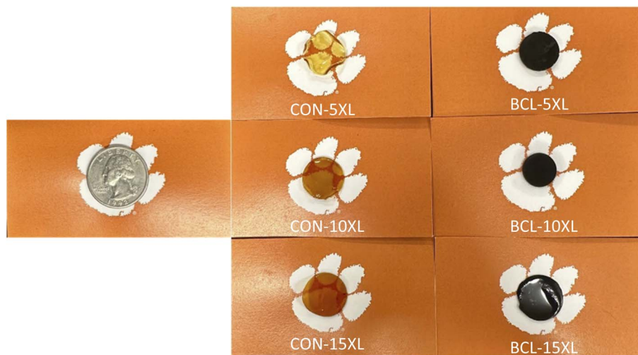
Fig. 3 Images of the hydrated, free-standing PNIPAm–PVA control (CON) hydrogel membranes and lignin–PNIPAm–PVA biocomposite hydrogel membranes containing BioChoice lignin (BCL). In each column, the crosslinker concentration increases progressively from 5 to 15 mass%, moving from top to bottom. Note that the diameter of a United States quarter is approximately 25 mm.
