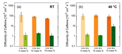
Fig. 6 Caffeine diffusivity for PNIPAm-PVA control (CON) hydrogel membranes and lignin-PNIPAm-PVA biocomposite hydrogel membranes (BCL) at (a) RT and (b) 40 °C. The error bars represent the standard deviation of the average diffusivity calculated from measurements on (at least) three separate membranes.
