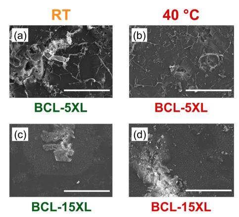
Fig. 9 SEM images of BCL hydrogels with 5 mass% crosslinker at (a) RT and (b) 40 °C and with 15 mass% crosslinker at (c) RT and (d) 40 °C. Note that the scale bar in all the images is 500  $\mu$ m.
