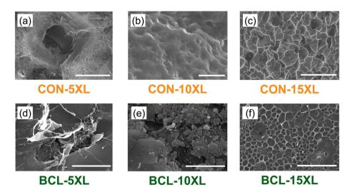
Fig. 7 SEM images of CON hydrogels at (a) 5 mass%, (b) 10 mass%, and (c) 15 mass% crosslinker, and BCL hydrogels at (d) 5 mass%, (e) 10 mass%, and (f) 15 mass% crosslinker. All hydrogels were hydrated in water at room temperature. Note that the scale bar in all the images is 100 µm.
