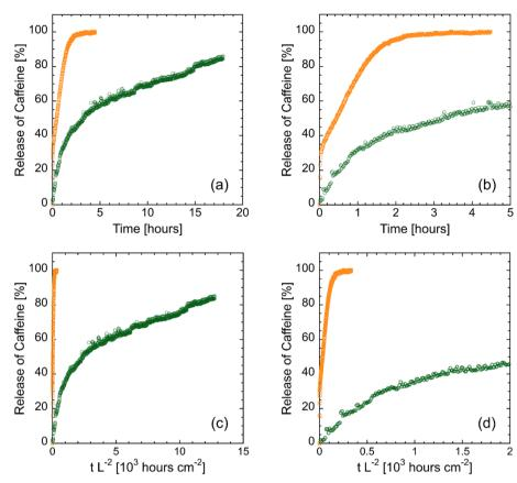
Fig. 5 Caffeine release profiles for a PNIPAm–PVA control (CON, orange squares) hydrogel membrane and a lignin–PNIPAm–PVA biocomposite hydrogel membrane (BCL, green circles) at 15 mass% crosslinker and RT for (a) up to 18 hours, (b) the first hour, (c) the release profile normalized by thickness, centered for the BCL hydrogel profile, and (d) the release profile normalized by thickness, enlarged to capture the CON hydrogel profile.
