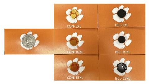
Fig. 3 Images of the hydrated, free-standing PNIPAm-PVA control (CON) hydrogel membranes and lignin-PNIPAm-PVA biocomposite hydrogel membranes containing BioChoice lignin (BCL). In each column, the crosslinker concentration increases progressively from 5 to 15 mass%, moving from top to bottom. Note that the diameter of a United States quarter is approximately 25 mm.
