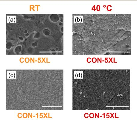
Fig. 8 SEM images of CON hydrogels with 5 mass% crosslinker at (a) RT and (b) 40 °C and with 15 mass% crosslinker at (c) RT and (d) 40 °C. Note that the scale bar in all the images is 500 µm.
