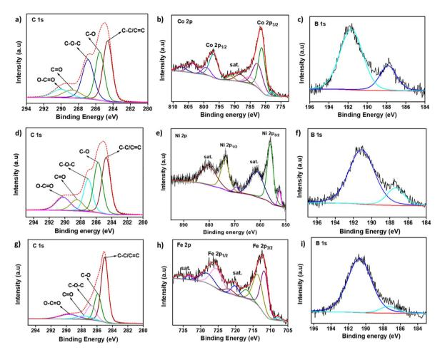
Fig. 4 XPS spectra of (a) C 1s, (b) Co 2p, and (c) B 1s for ON10/Co-B. XPS spectra of (d) C 1s, (e) Ni 2p and (f) B 1s for ON10/Ni-B. XPS spectra of (q) C 1s, (h) Fe 2p and (i) B 1s for ON10/Fe-B.
