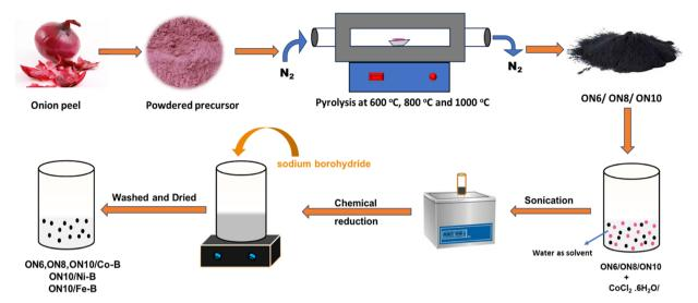
Schematic of the synthesis of carbon and carbon-supported transition metal borides
