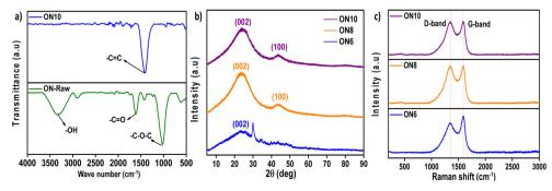
Fig. 2 (a) FTIR spectra of ON-raw and ON10. (b) XRD pattern and (c) Raman spectra of ON6, ON8, and ON10.
