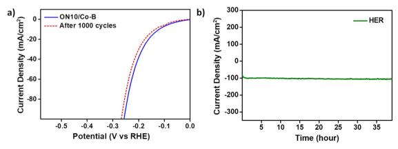
Fig. 6 (a) Linear polarization curves for the HER before and after 1000 cycles. (b) Chronoamperometric plot of ON10/Co-B for 40 h.
