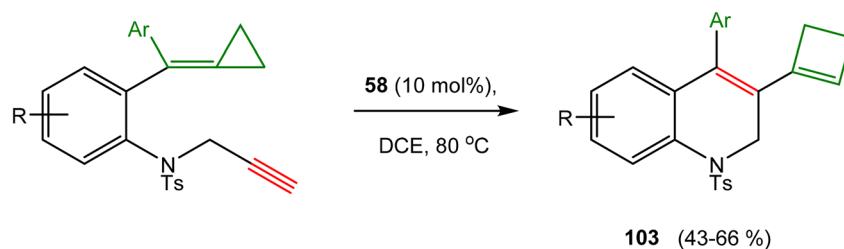
Scheme 41 NHC-gold-catalyzed intramolecular annulation of aniline-linked 1,7-enynes.
