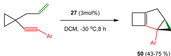
Scheme 21 Cycloisomerization of 1,5-enynes, catalyzed by the NHC-Au(I)-NTf 2 complex 27 .
