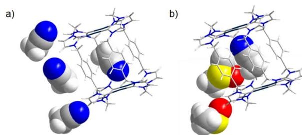
**Fig. 5** Orientation of the acetonitrile molecule (space-filling model) trapped inside the hollow cavity of box-like complex cation  $[Ag_4(1)_2]^{4+}$ : (a) obtained through diethyl ether diffusion into pure acetonitrile; (b) obtained through diethyl ether diffusion into DMSO/acetonitrile. Tetraphenylborate anions are omitted for clarity.
