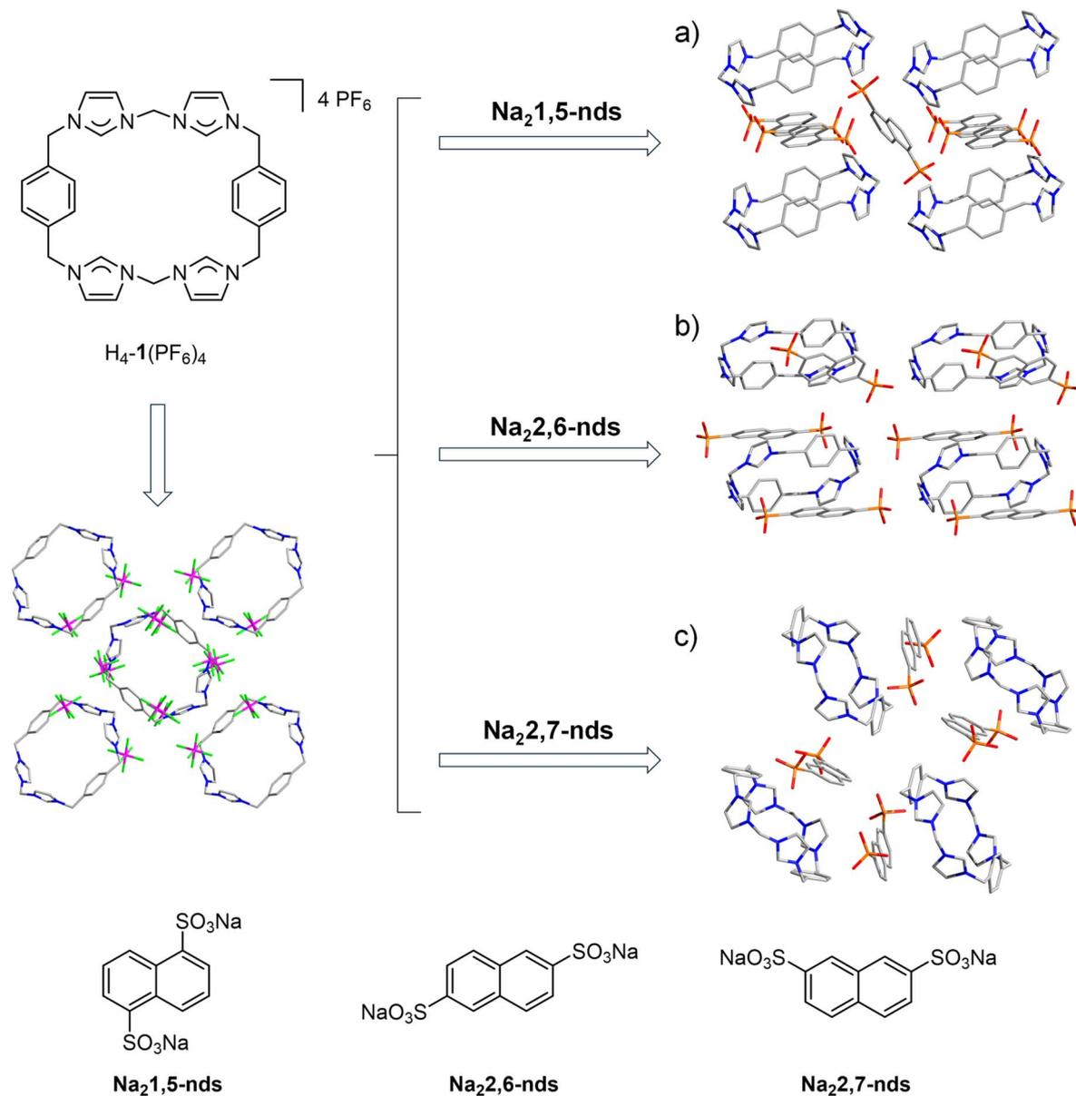
Fig. 3 Anion exchange in the macrocyclic complex  $H_4-1(PF_6)_4$  with naphthalene disulfonate ( $Na_2nds$ ) and crystal packing diagrams of (a)  $[H_4-1(1,5-nds)_2]$ , (b)  $H_4-1(2,6-nds)_{1.5}$  and (c)  $[H_4-1(2,7-nds)_2]$  (hydrogen atoms,  $CH_3CN$  and  $H_2O$  molecules omitted for clarity).
