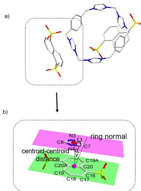
Fig. 2 (a) The binding mode between  $(H_4-1)$  and 1,5-naphthalene disulfonate dianion (1,5-nds) in stick form. (b) Expanded  $\pi$ - $\pi$  donor-acceptor interaction stacking part in stick form. All the other molecules and atoms have been omitted for clarity. The possible  $\pi$ - $\pi$  interactions were inferred from the following selected.
