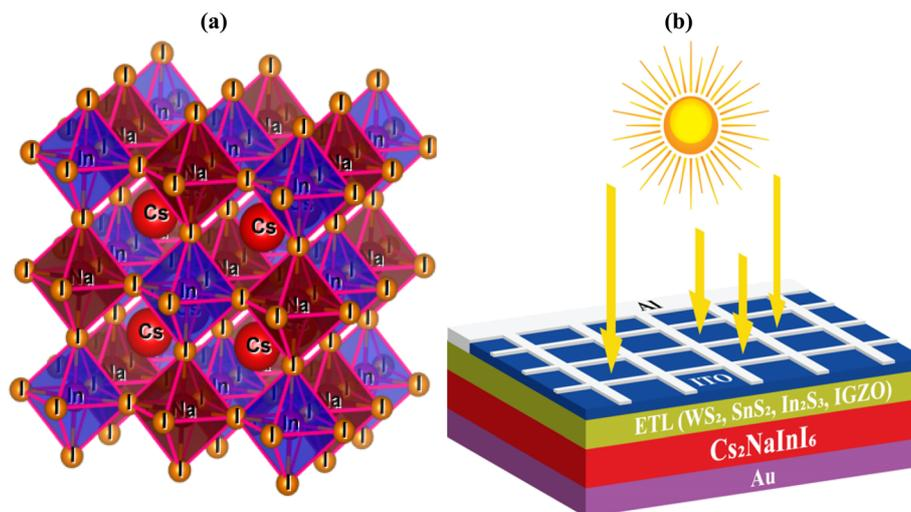
Fig. 1 (a) Crystal structure of the  $\text{Cs}_2\text{NaInI}_6$ , and (b) device architecture of the  $\text{Cs}_2\text{NaInI}_6$ -based PSC.
