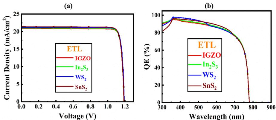
Fig. 8 (a)  $J$ - $V$ , (b) QE curve with various ETL of  $\text{Cs}_2\text{NaInI}_6$ -based double PSC.
