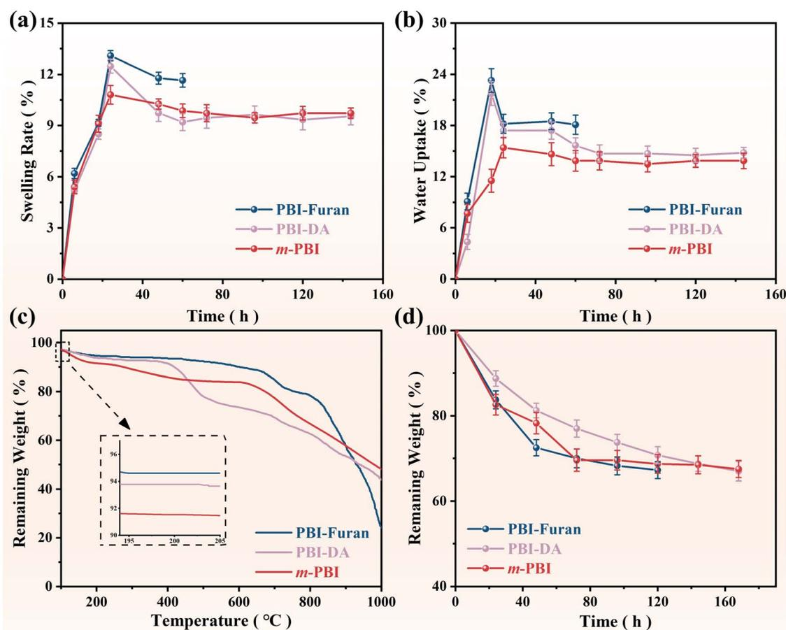
**Fig. 5** (a) Water uptake and (b) swelling ratio at 80 °C of PBI-furan, PBI-DA and *m*-PBI. (c) The remaining weight from TG of PBI-furan, PBI-DA and *m*-PBI. Test conditions: room temperature ~1000 °C, nitrogen atmosphere, heating rate: 10 °C min<sup>-1</sup>. (d) The antioxidant stability curves of PBI-furan, PBI-DA and *m*-PBI. Test conditions: Fenton reagent (4 ppm Fe<sup>2+</sup>, 3% H<sub>2</sub>O<sub>2</sub>, incubated at 70 °C for 24 h).
