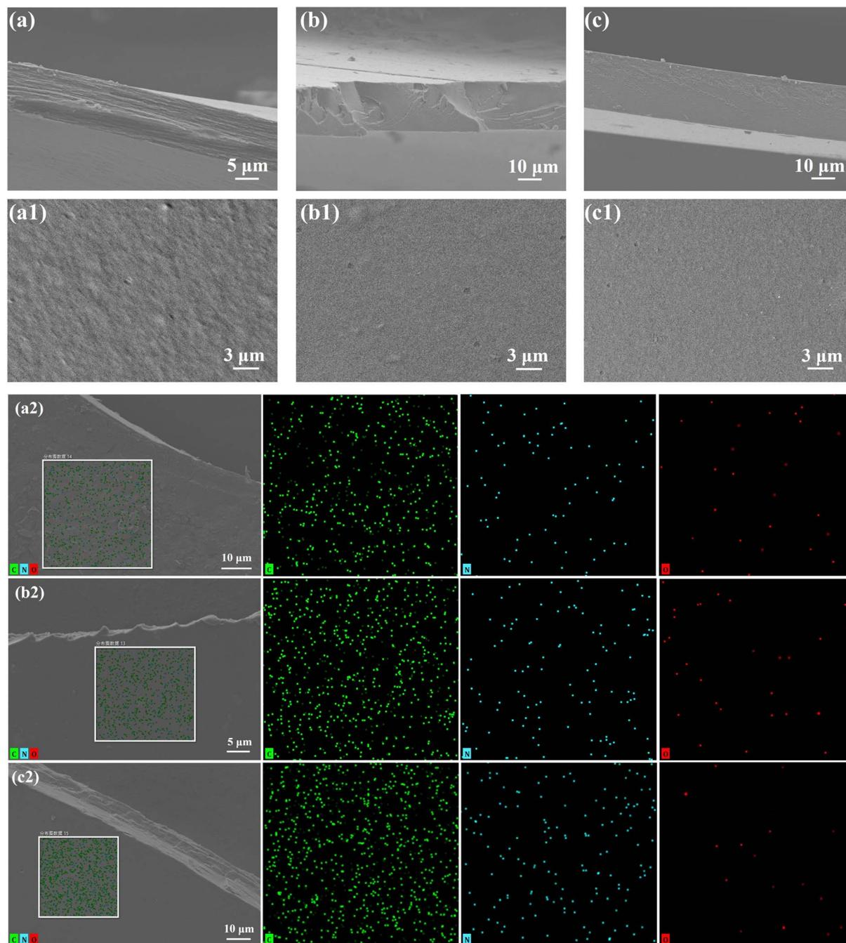
**Fig. 2** The cross-sectional SEM images of (a) PBI-furan, (b) PBI-DA and (c) *m*-PBI (treated with Pt coating after fractured in liquid nitrogen). The surface SEM image of (a1) PBI-furan, (b1) PBI-DA and (c1) *m*-PBI (treated with Pt coating after fractured in liquid nitrogen). The distribution of C, N, O element from EDS maps of (a2) PBI-furan, (b2) PBI-DA and (c2) *m*-PBI.
