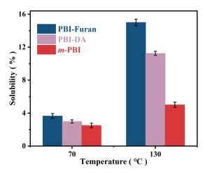
Fig. 3 The solubility of PBI-furan, PBI-DA and m-PBI in NMP at different temperatures.
