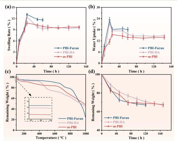
Fig. 5 (a) Water uptake and (b) swelling ratio at 80 °C of PBI-furan, PBI-DA and m-PBI. (c) The remaining weight from TG of PBI-furan, PBI-DA and m-PBI. Test conditions: room temperature  $\sim$ 1000 °C, nitrogen atmosphere, heating rate: 10 °C min<sup>-1</sup>. (d) The antioxidant stability curves of PBI-furan, PBI-DA and m-PBI. Test conditions: Fenton reagent (4 ppm Fe<sup>2+</sup>, 3% H<sub>2</sub>O<sub>2</sub>, incubated at 70 °C for 24 h).
