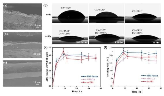
Fig. 4 The cross-sectional SEM images of (a) PBI-furan, (b) PBI-DA and (c) m-PBI all doped with phosphate acid (fractured in liquid nitrogen). (d) Phosphate acid contact angle of different polymer membranes at 0 s and 30 s. (e) ADL and (f) swelling ratio of PBI-furan, PBI-DA and m-PBI in phosphoric acid.
