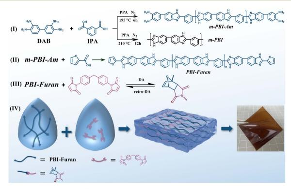
Scheme 1 Synthesis route of the polymers: (I) low molecular weight m-PBI Am and m-PBI as the control group. (II) Furan-capped prepolymer (PBI-furan). (III) Chain extended polymer (PBI-DA). (IV) Solution pouring and preparation for film formation.
