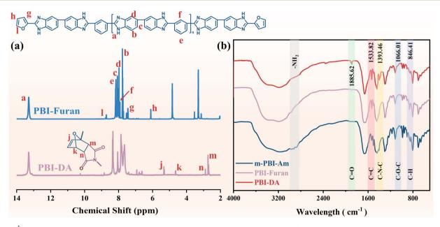
Fig. 1 (a) <sup>1</sup>H NMR spectra of prepolymer PBI-furan and chain-extended polymer PBI-DA. (b) FT-IR spectra of prepolymer PBI-furan, chain-extended polymer PBI-DA and *m*-PBI-Am.
