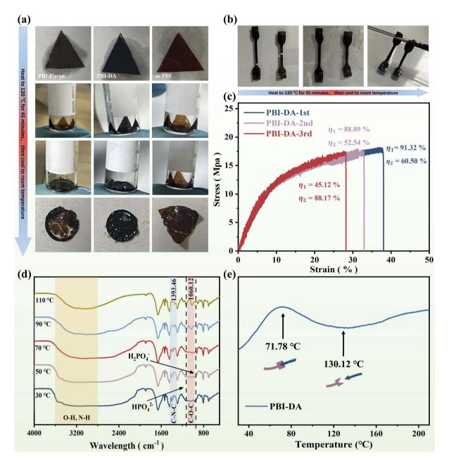
Fig. 7 (a) Melting behavior of phosphoric acid doped membranes at high temperature. (b) Self-healing behavior of PBI-DA spline at 120 °C. (c) Mechanical strength of self-healed PBI-DA spline. (d) The temperature dependent FT-IR spectrum of phosphoric acid doped PBI-DA membrane. (e) The DSC curve of PBI-DA membrane.
