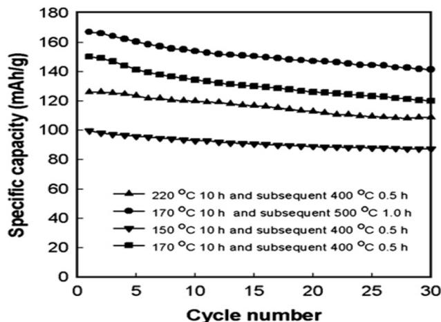
Fig. 5 Cycling stability of  $\text{LiFePO}_4$  prepared at different temperatures.<sup>60</sup> This figure is adopted/reproduced/reprinted from ref. 60 with agreement from Elsevier, copyright 2007.
