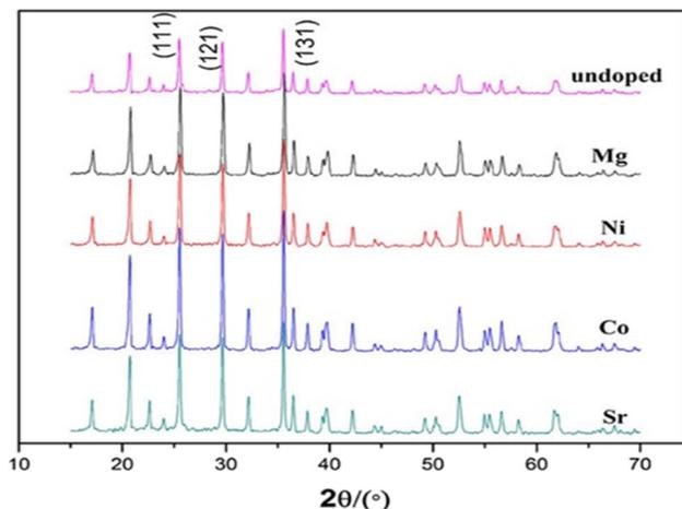
Fig. 16 XRD patterns of LFP samples doped with different metal ions.<sup>106</sup> Reproduced from ref. 106 with permission from the John Wiley and Sons, copyright 2013.
