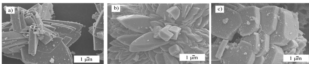
Fig. 4 FE-SEM micrographs of LFP powders prepared hydrothermally for 12 h with 20 mmol urea and  $\text{Li}_2\text{SO}_4$  (Li : Fe : P = 3 : 1 : 1) at different temperatures:  $170^\circ\text{C}$  (a),  $180^\circ\text{C}$  (b),  $190^\circ\text{C}$  (c).<sup>57</sup> This figure is adopted/reproduced/reprinted from ref. 57 with agreement from Elsevier, copyright 2017.
