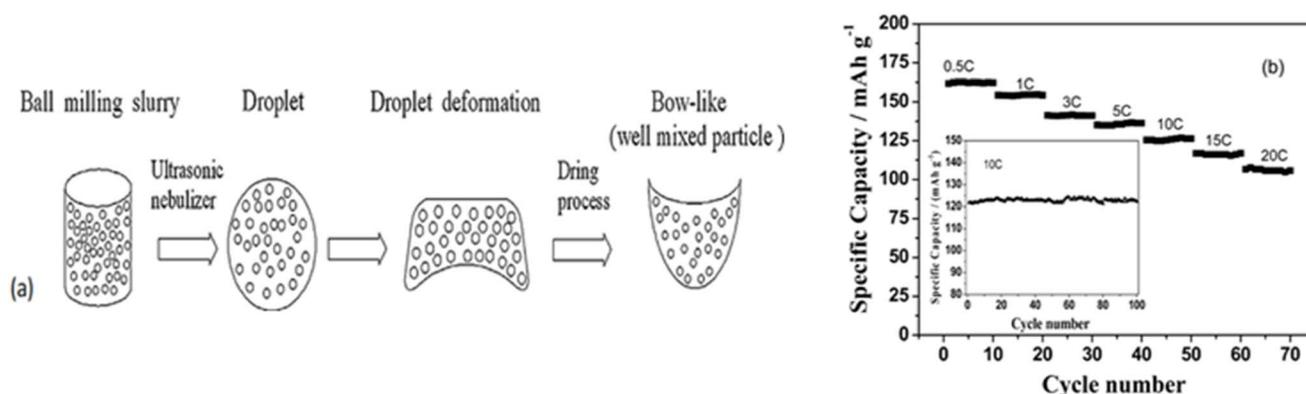
Fig. 8 (a) Formation scheme of the mesoporous bowl-like LiFePO<sub>4</sub>/C morphology and (b) its discharge profiles and rate capability at different current densities.<sup>66</sup> This figure being adopted/reproduced/reprinted from ref. 66 with permission from Elsevier, copyright 2003.
