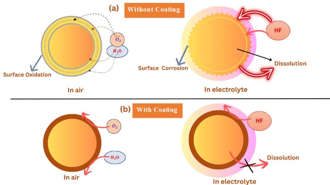
Fig. 10 Schematic illustration of cathode behavior with (b) and without carbon coating (a).
