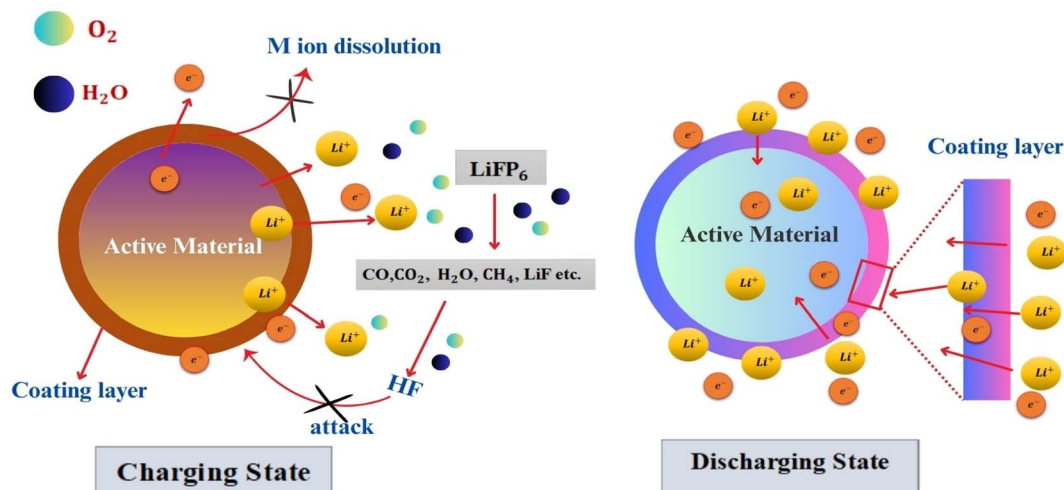
Fig. 3 Effect of surface coating on cathode materials in suppressing side reactions and enhancing structural stability.
