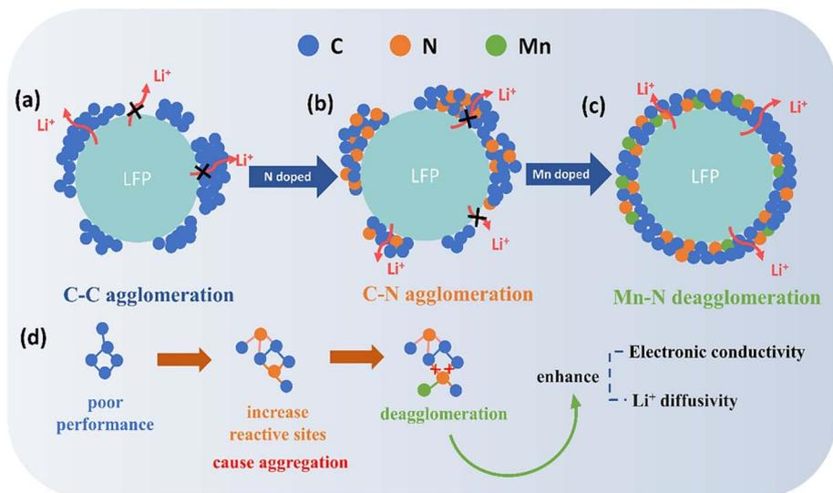
Fig. 13 (a) Carbon coating on LFP; (b) layer of N-doped carbon on LFP; (c) N–Mn co-doped carbon layer on LFP; and (d) Mn-induced deagglomeration effect.<sup>38</sup> Reproduced from ref. 38 with permission from the American Chemical Society, copyright 2024.
