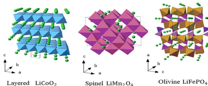
Fig. 2 Crystal structures of layered  $\text{LiCoO}_2$ , spinel  $\text{LiMn}_2\text{O}_4$  and olivine  $\text{LiFePO}_4$  cathode materials.<sup>9,10</sup> Reproduced from open access article ref. 9 with permission MDPI, copyright 2014.
