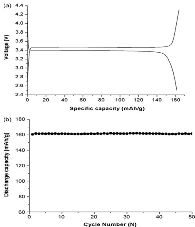
Fig. 6 (a) Charge–discharge curve and (b) cycling performance of  $\text{LiFePO}_4/\text{C}$  (8.10 : 1 ball milling, 2 min microwave) at 27 °C.<sup>63</sup> This figure is adopted/reproduced/reprinted from ref. 63 with permission from Elsevier, copyright 2007.
