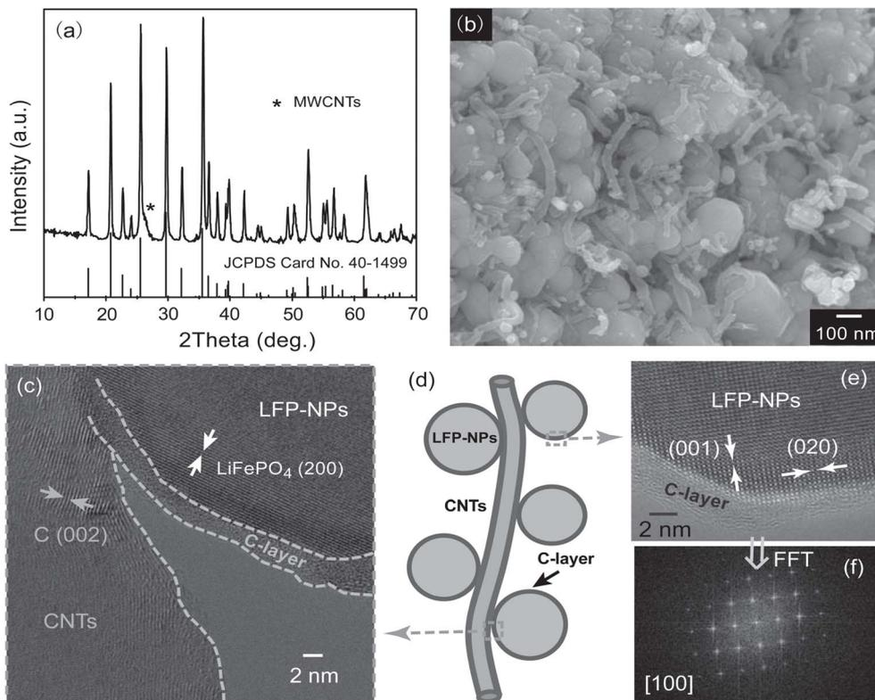
Fig. 17 (a) XRD pattern, (b) SEM, (c and e) HRTEM images, (d) schematic illustration of the generated LFP@C/CNT nanocomposite, and (f) the corresponding FFT from the HRTEM in (e).<sup>122</sup> Reproduced from ref. 122 with permission from John Wiley and Sons, copyright 2013.
