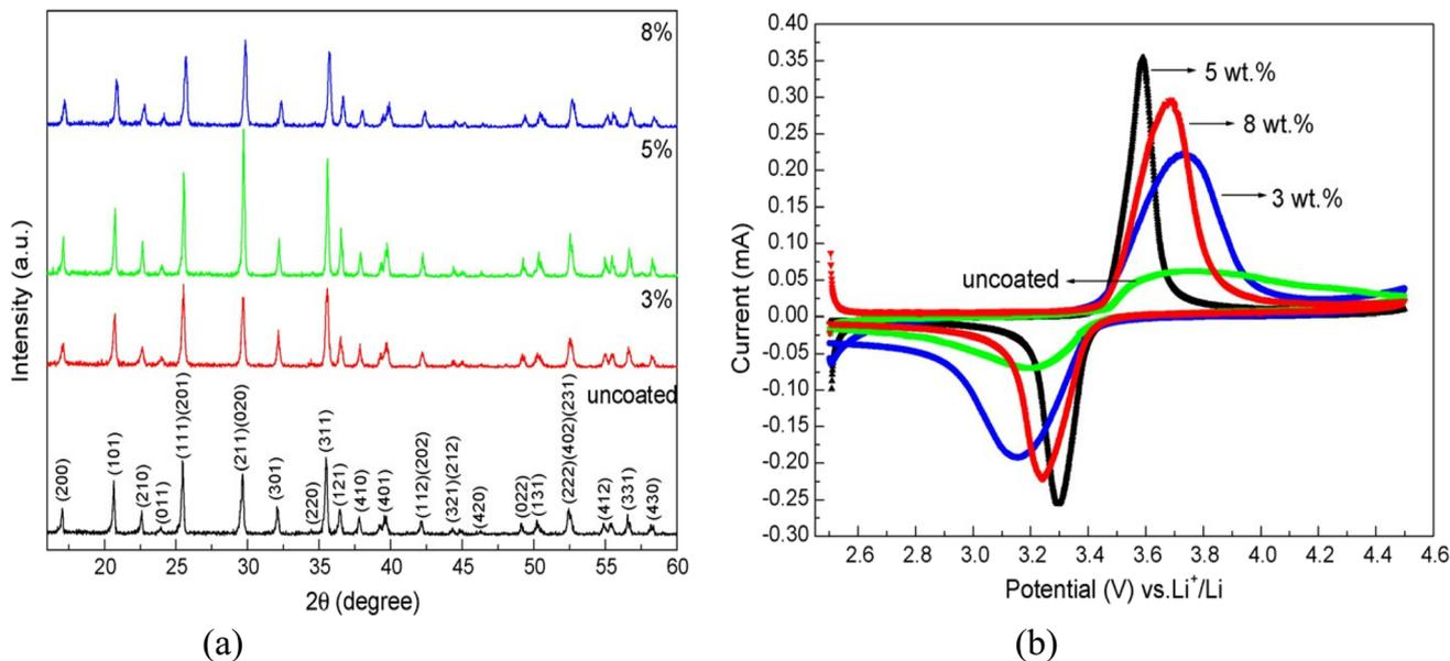
Fig. 11 Comparison of the XRD patterns (a) and cyclic voltammetry profiles (b) of the uncoated LFP and LFP/MWCNT composites.<sup>95</sup> Both figures (a and b) are reproduced from ref. 95 with permission from Elsevier, copyright 2009.
