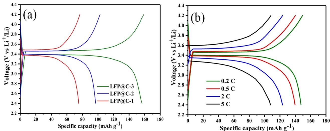
Fig. 9 (a) Initial charge–discharge profiles of synthesized electrode materials at 0.1C and (b) charge–discharge profile of LFP@C-3 at different rates of 0.2C, 0.5C, 2C and 5C.<sup>72</sup> This figure is reproduced from ref. 72 with the permission from Elsevier, copyright 2019.
