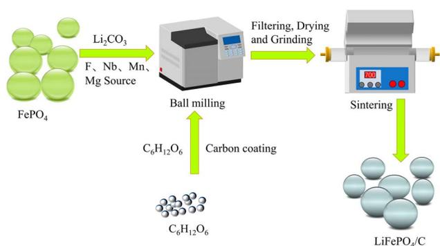
Fig. 15 Schematic representation of the carbothermal reduction process paired with a combined bulk phase doping approach to prepare LFP/C cathode materials.<sup>98</sup> Reproduced from open access article ref. 98 with permission MDPI, copyright 2024.
