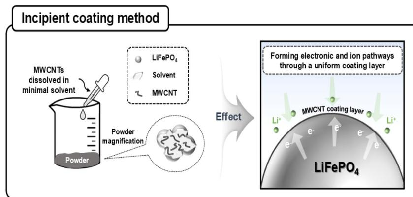
Fig. 12 Incipient coating of MWCNTs on LFP enhances electron and ion pathways.<sup>96</sup> Reproduced from ref. 96 with permission from the American Chemical Society, copyright 2025.
