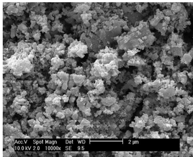
Fig. 7 SEM Analysis of  $\text{LiFePO}_4$  particles synthesized by microwave heating for 4 minutes.<sup>64</sup> This figure is adopted/reproduced/reprinted from ref. 64 with permission from Elsevier, copyright 2003.
