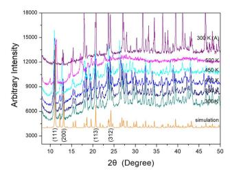
Fig. 4 Powder X-ray diffraction (PXRD) patterns with temperature variation and the simulated XRD pattern of  $[N(C_2H_5)_4]_2CdBr_4$ . The 300 K (A) pattern represents the PXRD pattern measured after cooling the single crystal from 500 K to 300 K.
