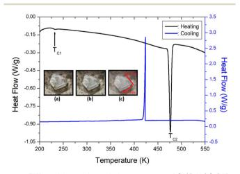
Fig. 1 Differential scanning calorimetry curves of  $[N(C_2H_5)_4]_2CdBr_4$  measured at a heating and cooling rate of 10 K min<sup>-1</sup> (inset: single crystal images at (a) 300 K, (b) 513 K, and (c) 583 K).
