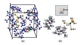
Fig. 3 (a) Tetragonal structure and (b) thermal ellipsoids for two type of  $[N(C_2H_5)_4]$  cations and  $CdBr_4$  anion of  $[N(C_2H_5)_4]_2CdBr_4$  crystal at 300 K (inset: morphology of a colorless and transparent single crystal at 300 K) (CCDC no. 2477720).
