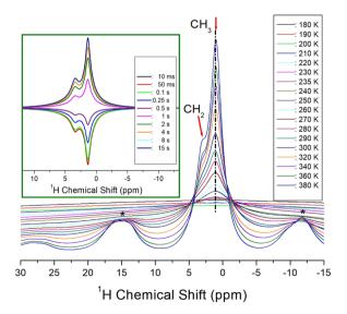
Fig. 5  $^{1}$ H NMR spectra for CH<sub>2</sub> and CH<sub>3</sub> in [N(C<sub>2</sub>H<sub>5</sub>)<sub>4</sub>]<sub>2</sub>CdBr<sub>4</sub> with increasing temperature (inset: recovery traces measured with the delay time of 10 ms–15 s).
