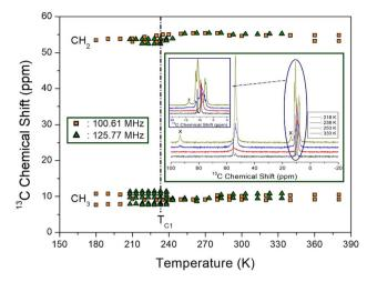
Fig. 6  $^{13}$ C NMR chemical shifts for CH<sub>2</sub> and CH<sub>3</sub> in [N(C<sub>2</sub>H<sub>5</sub>)<sub>4</sub>]<sub>2</sub>CdBr<sub>4</sub> measured at Larmor frequency of 100.61 and 125.77 MHz with increasing temperature (inset:  $^{13}$ C NMR spectra at 218, 238, 253, and 333 K)
