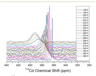
Fig. 8  $^{113}$ Cd NMR spectra in  $[N(C_2H_5)_4]_2$ CdBr $_4$  with increasing temperature.
