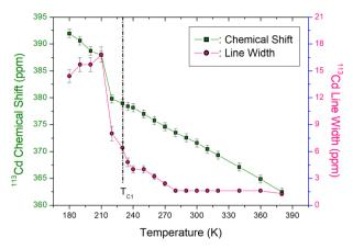
Fig. 9  $^{113}$ Cd NMR chemical shifts and line widths in  $[N(C_2H_5)_4]_2$ CdBr<sub>4</sub> near the phase transition temperature  $T_{C1}$ .
