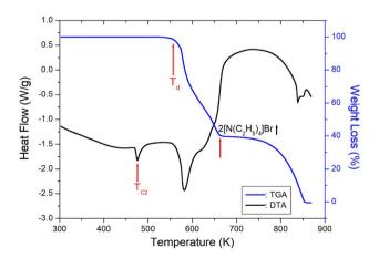
Fig. 2 Thermogravimetry and differential thermal analysis curves of  $[N(C_2H_5)_4]_2CdBr_4$  measured at a heating rate 10 K min<sup>-1</sup>.  $T_d$  is the decomposition temperature.
