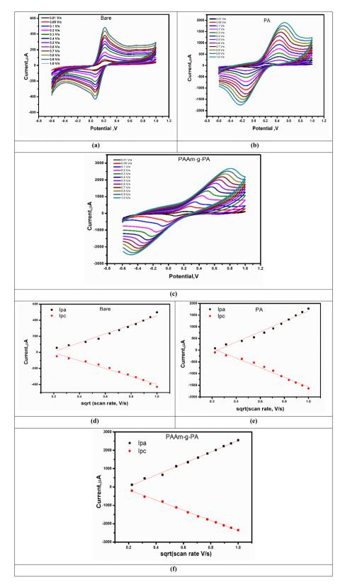
Fig. 4 CV data illustrated the effect of scan rate on the FCN redox reactions at modified SPCEs. Continuous rise in the currents of oxidation–reduction peak as the scan rate rose for (a) the unmodified (bare), (b) PA, and (c) PAAm-g-PA. The relationship between the current and the scan rates square roots of (d) unmodified (bare), (e) PA, and (f) PAAm-g-PA.
