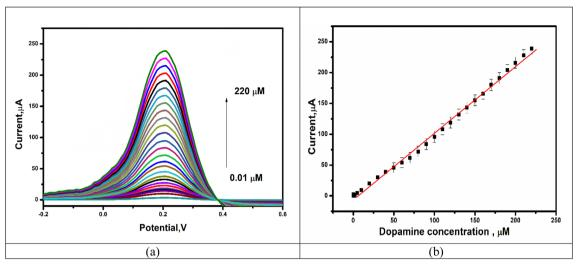
Fig. 7 (a) DPV curves for various DA levels (0.01–220 μM) in PBS at pH 7.5 using PAAm-g-PA/SPCE. (b) Calibration curves of various DA concentrations via peak current.
