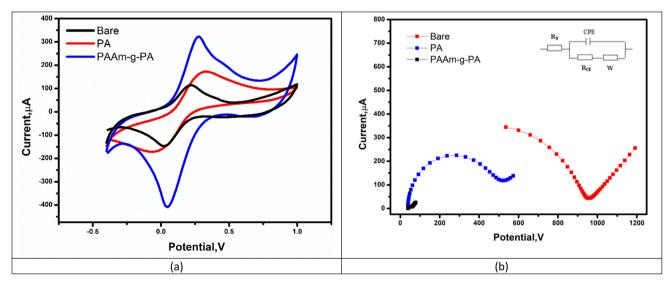
Fig. 3 (a) CV and (b) EIS (the figure inset depicts the circuit that was utilized to fit the EIS data). For bare (unmodulated), PA, beside PAAm-g-PA/ SPCE in a solution containing 5 mM [Fe(CN) $_6$ ]<sup>3-/4-</sup>, with a scan rate of 50 mV s<sup>-1</sup> for cyclic voltammetry measurements.
