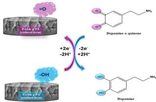
Scheme 2 DA redox reaction mechanism
