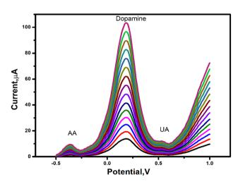
Fig. 9 DPV responses for varied DA concentrations with varying AA and UA concentrations in PBS at pH 7.5, using the PAAm-*q*-PA/SPCE.
