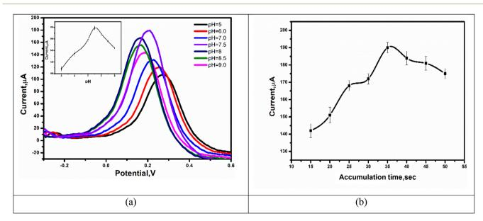
Fig. 6 (a) DPV and pH values bar diagram against the peak of electrical current (inset figure) for 180  $\mu$ M of DA in PBS at pH 7.5 with a deposition time of 35 seconds, beside a scan rate of 50 mV s<sup>-1</sup>. (b) Time of accumulation against the electrical current response in PBS at pH 7.5 with 180  $\mu$ M of DA at a scan rate of 50 mV s<sup>-1</sup>.
