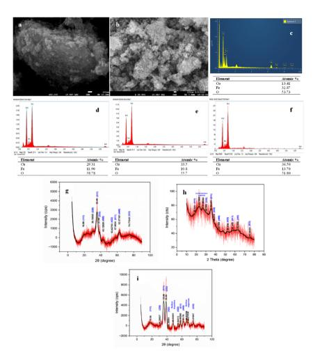
Fig. 5 (a) SEM of fresh catalyst; (b) SEM of recycled catalyst; (c) EDX of small spherical domain (fresh); (d) EDX of large domain (fresh); (e) EDX of small spherical domain (recycled); (f) EDX of large domain (recycled); (g) PXRD of fresh catalyst; (h) PXRD of recycled catalyst after 5 cycles without calcination; (i) PXRD of recycled catalyst after calcination at 400 °C for 2 h.
