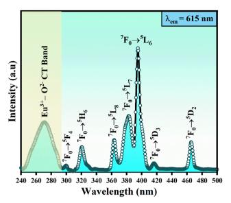
Fig. 4 Excitation spectrum corresponding to the  $\beta$ -BaB<sub>2</sub>O<sub>4</sub>:xEu<sup>3+</sup> (x = 2 mol%) phosphors.
