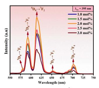
Fig. 5 PL emission spectra for  $\beta\text{-BaB}_2\text{O}_4\text{:}x\text{Eu}^{3+}$  with excitation at 395 nm.
