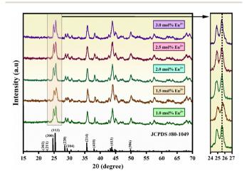
Fig. 1 Experimental XRD patterns overlaid with standard reference peaks confirming the crystalline phase of the phosphors.
