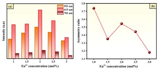
Fig. 7 (a) Variation of intensity for the peaks at 593, 615, and 702 with the concentration of Eu<sup>3+</sup>. (b) Concentration dependent asymmetry ratio.
