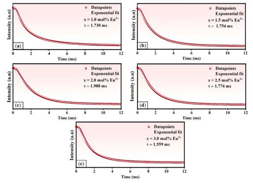
(a)-(e) Decay curves corresponding to the doped phosphors.
