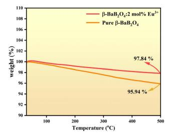
Fig. 13 TGA curve for  $\beta$ -BaB<sub>2</sub>O<sub>4</sub>:xEu<sup>3+</sup> (x = 2 mol%) phosphor.
