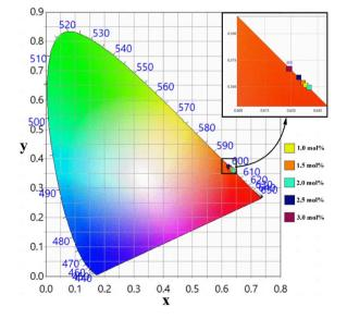
Fig. 10 Chromaticity coordinates of the synthesized phosphors in the CIE 1931 colour coordinate diagram.
