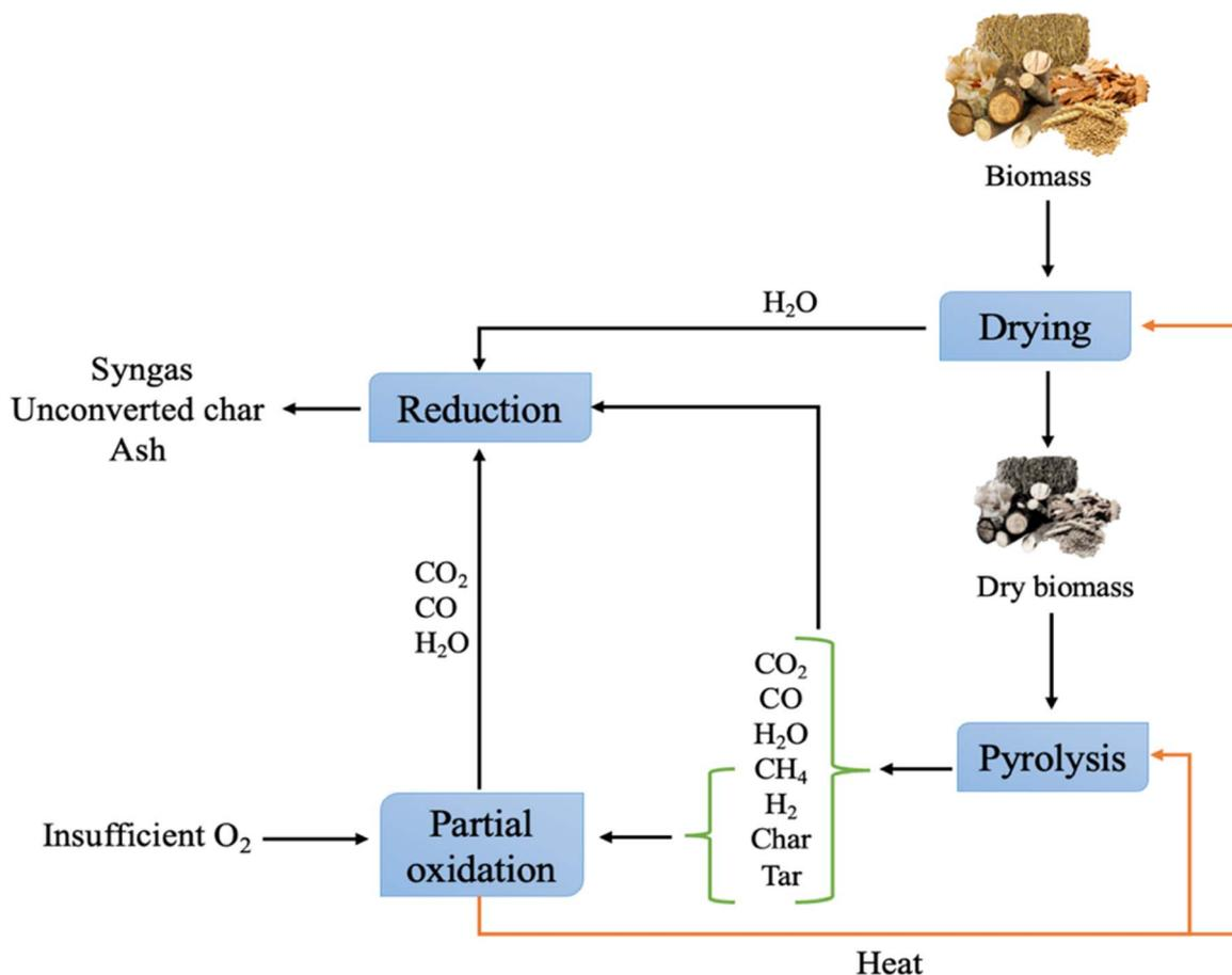
Fig. 10 Main reactions in the gasification of biomass.
