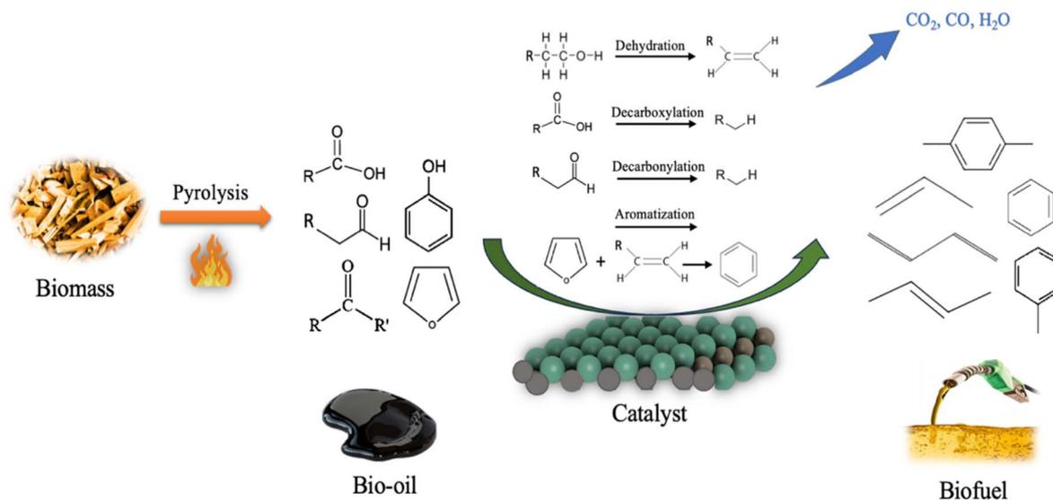
Fig. 16 Major reaction pathways for bio-oil catalytic upgrading.
