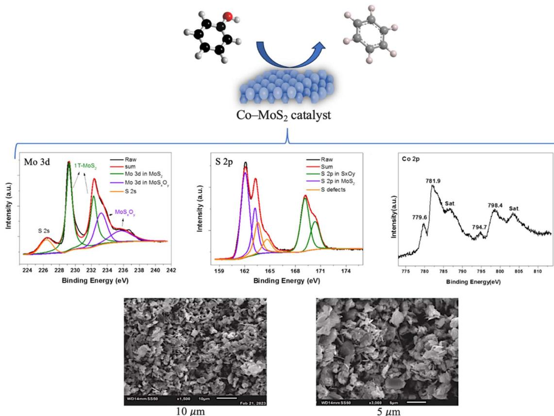
Fig. 17 XPS spectra and SEM images of the Co-MoS<sub>2</sub> catalyst, adapted from ref. 206 with permission from Elsevier, *Case Studies in Chemical and Environmental Engineering*, vol. 9, p. 100734, Copyright 2024.
