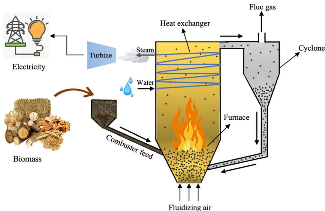
Fig. 15 Schematic of a typical CFBC system.
