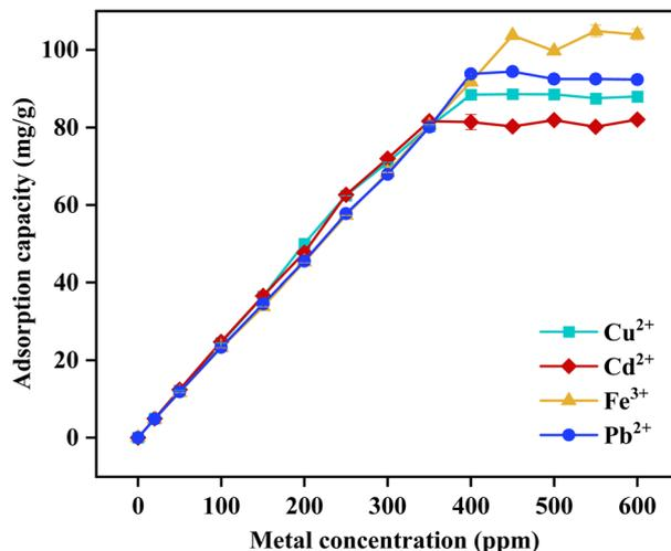
Fig. 16 Effect of the initial metal concentration on the adsorption capacity of PBC 150/1.0/9 (adsorption conditions: dosage 0.04 g/10 mL, temperature 30 °C, time 120 min, pH  $5.0 \pm 0.2$ , for  $\text{Fe}^{3+}$  pH 2.5).
