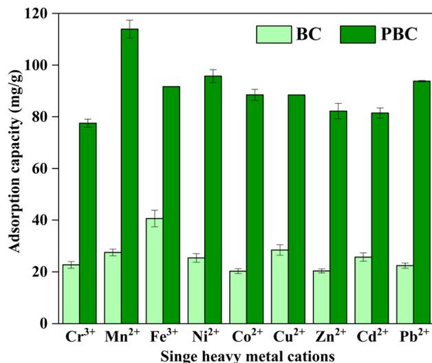
Fig. 19 Single-metal ion adsorption of BC and PBC 150/1.0/9 (adsorption conditions: dosage 0.04 g/10 mL, concentration 400 ppm, temperature 30 °C, time 120 min, pH 5.0 ± 0.2, for Fe<sup>3+</sup> pH 2.5).
