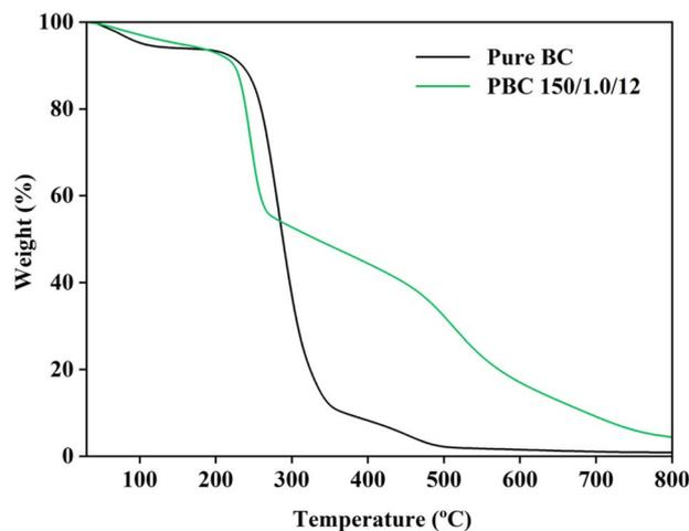
Fig. 7 TGA profiles of pure BC and PBC 150/1.0/12.
