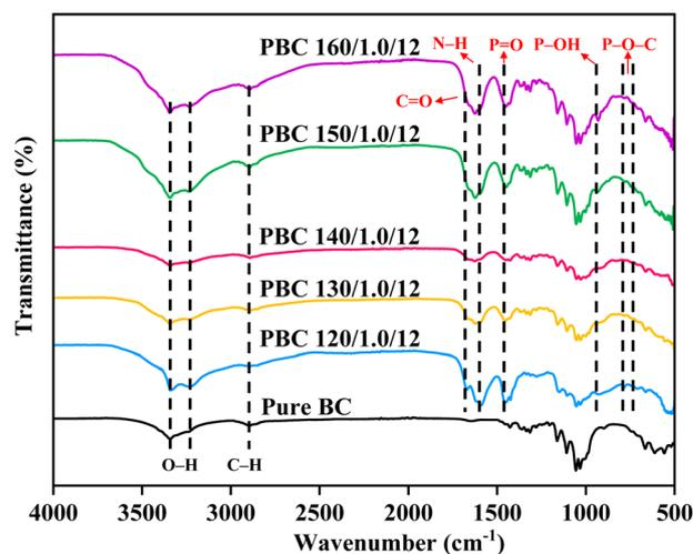
Fig. 6 FTIR spectra of pure BC and PBC.
