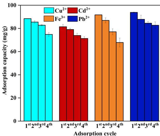
Fig. 21 Recycling tests for PBC 150/1.0/9 (adsorption conditions: dosage 0.04 g/10 mL, concentration 400 ppm, temperature 30 °C, time 120 min, pH 5.0 ± 0.2, for Fe<sup>3+</sup> pH 2.5).
