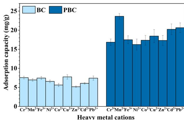
Fig. 20 Multi-metal ions adsorption of BC and PBC 150/1.0/9 (adsorption conditions: dosage 0.04 g/10 mL, concentration 50 ppm, temperature 30 °C, time 120 min, pH 3.0 ± 0.2).
