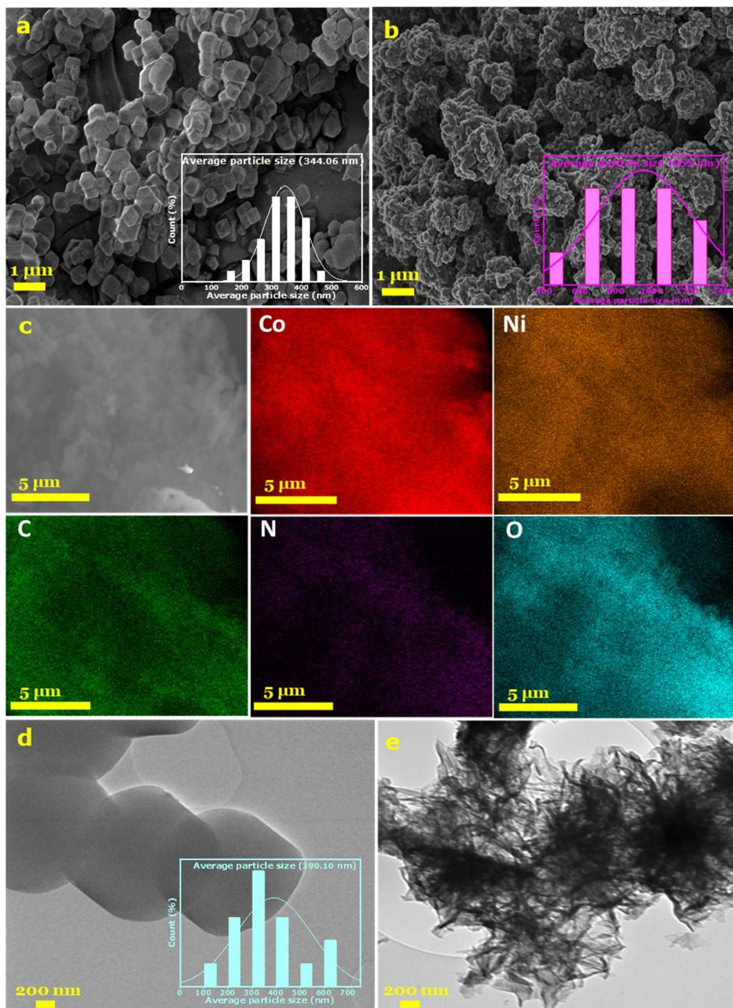
Fig. 2 SEM images at low magnification of (a) ZIF-67 and (b) ZIF-67 : Ni (1 : 2), TEM images of (c) ZIF-67 and (d) ZIF-67 : Ni (1 : 2) and (e) EDX mapping showing the elemental distribution of Co, Ni, C, N and O of ZIF-67 : Ni (1 : 2).
