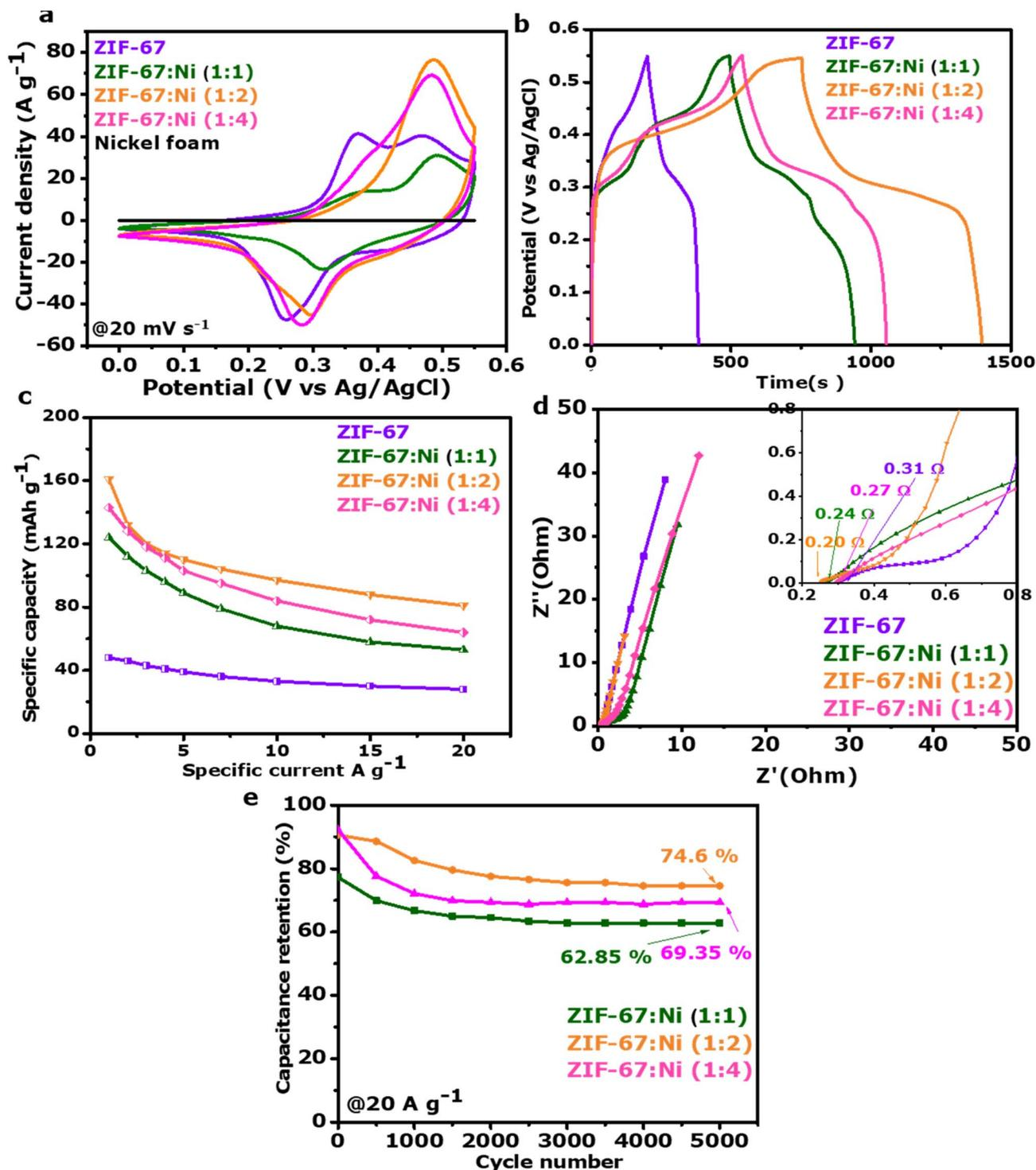
Fig. 6 (a) CV curves of the different electrodes at  $20 \text{ mV s}^{-1}$ , (b) GCD curves of the different electrodes at  $1 \text{ A g}^{-1}$ , (c) specific capacity against specific current of the different electrodes, (d) Nyquist plot of the different electrodes (inset shows the magnified plot) and (e) capacity retention of ZIF-67 : Ni (1 : X) up to 5000 cycles at a constant specific current at  $20 \text{ A g}^{-1}$ .
