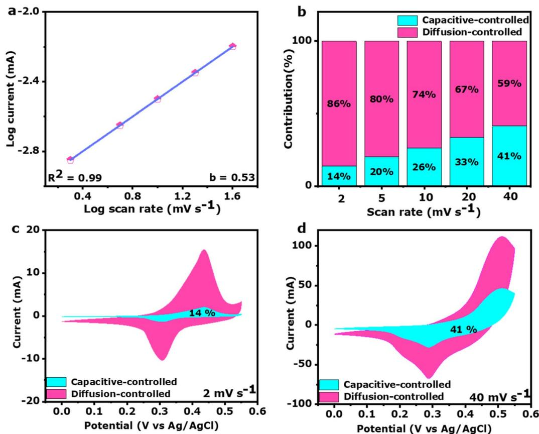
Fig. 7 (a) Linear plot of  $\log i(V)$  vs.  $\log \nu$ , (b) comparison of the contributions of surface capacitive and diffusion processes, (c) percentage of the capacitive map of the CV curve at  $2 \text{ mV s}^{-1}$  and (d) percentage of the capacitive map of the CV curve at  $40 \text{ mV s}^{-1}$ .
