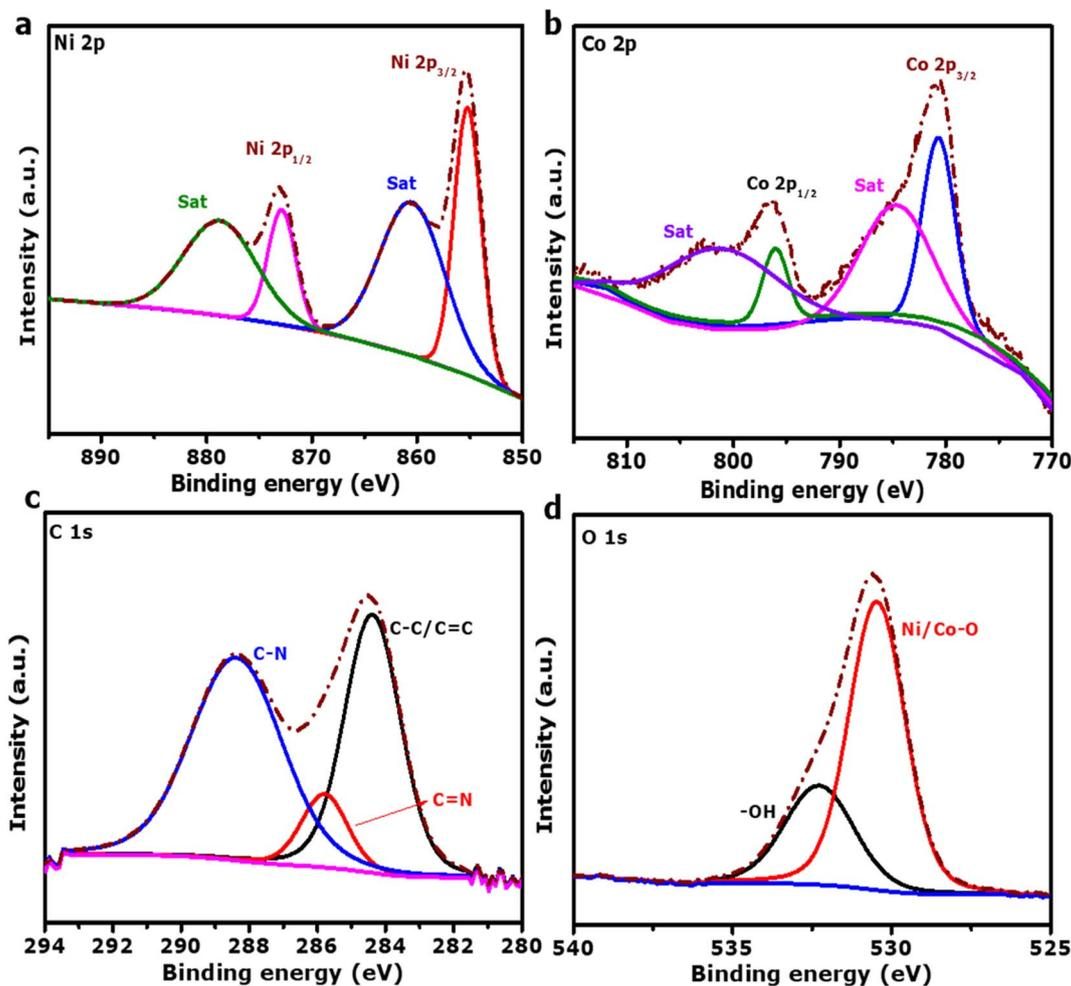
Fig. 4 (a) Deconvoluted XPS of Ni 2p, (b) Co 2p, (c) C 1s and (d) O 1s spectra of ZIF-67: Ni (1:2).
