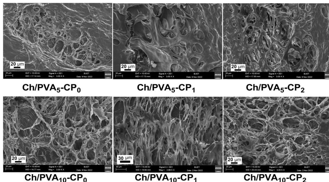
Fig. 5 SEM images of hydrogels for Ch/PVA<sub>5</sub> hydrogels (top row), Ch/PVA<sub>10</sub> (bottom row), and Ch: CP of 1:0, 1:1, and 1:2 combinations (arranged left to right, respectively). The images suggest a substantial degree of irregular crosslinking in the hydrogel. (Ch- Chitosan, CP- Collagen Peptide).
