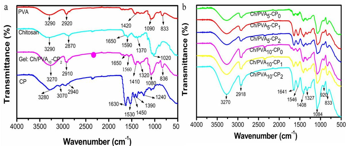
Fig. 2 (a) FTIR comparative spectra of PVA, chitosan, (Ch/PVA<sub>10</sub>-CP<sub>5</sub>) hydrogel, and collagen peptide (CP). Overlapping peaks from PVA, chitosan, and collagen peptide can be observed in the hydrogel spectrum. (b) FTIR spectra of various combinations of chitosan/PVA/collagen peptide. The spectra showed almost similar characteristic peaks for all hydrogels except for Ch/PVA<sub>5</sub>-CP<sub>0</sub> and Ch/PVA<sub>10</sub>-CP<sub>0</sub> (no amide peaks).
