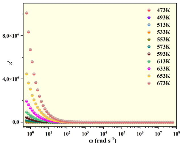
Fig. 8 Frequency dependence of  $\epsilon'$  at several temperatures.
