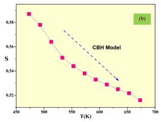
Fig. 3 (a) Frequency dependence of the ac conductivity at various temperatures. (b) Temperature dependence of the frequency exponent s
