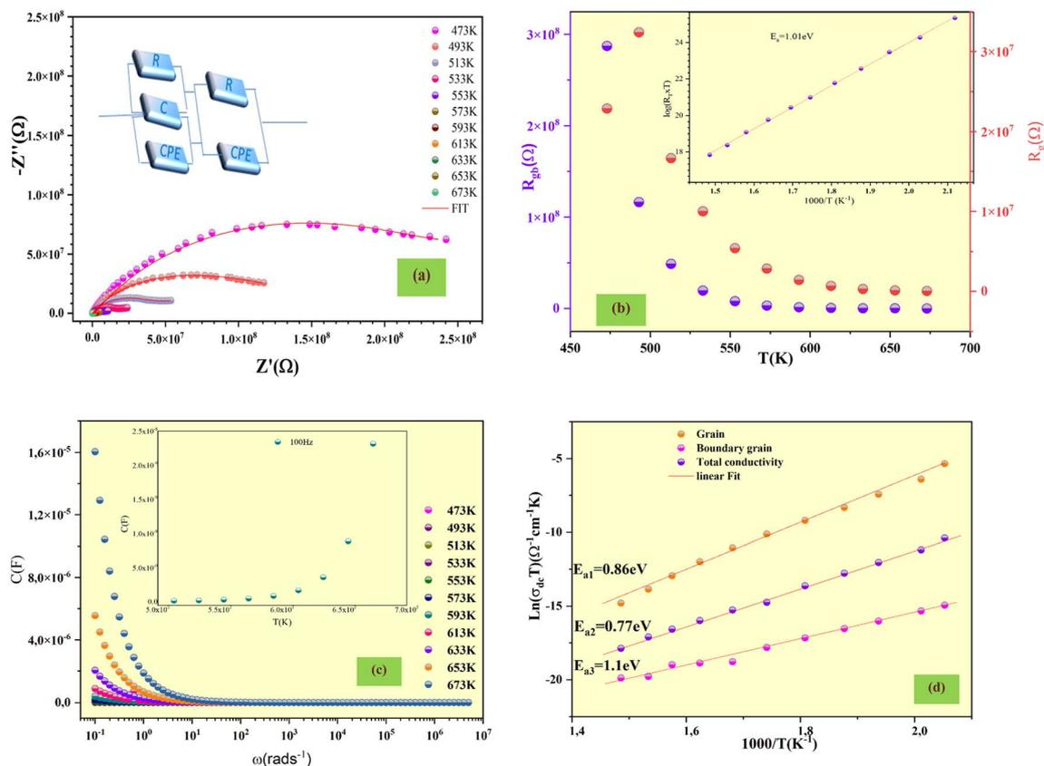
Fig. 2 (a) Nyquist plot with equivalent circuit representation of  $\text{LiVO}_3$ . (b) Temperature dependence of grain ( $R_g$ ) and grain boundary ( $R_{gb}$ ) resistances (inset: plot of  $\ln(R_{gb}/T)$  vs.  $1000/T$ ). (c) Frequency dependence of capacitance at different temperatures. (d) Variation of  $\ln(\sigma_{ac})$  as a function of temperature.
