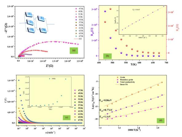
Fig. 2 (a) Nyquist plot with equivalent circuit representation of LiVO<sub>3</sub>. (b) Temperature dependence of grain ( $R_g$ ) and grain boundary ( $R_{gb}$ ) resistances (inset: plot of ln( $R_{gb}/T$ ) vs. 1000/T). (c) Frequency dependence of capacitance at different temperatures. (d) Variation of ln( $\sigma_{dc}$ ) as a function of temperature.
