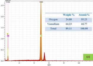
Fig. 1 (a) Powder X-ray diffractogram of LiVO<sub>3</sub> recorded at room temperature. The inset shows the crystal structure of the LiVO<sub>3</sub>. (b) Morphological analysis of LiVO<sub>3</sub> by SEM imaging. (c) Energy-dispersive X-ray (EDX) spectrum and elemental composition analysis.
