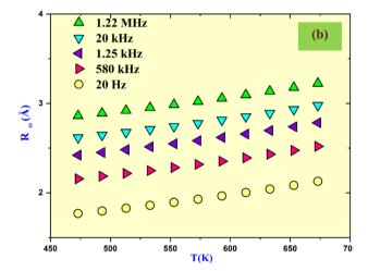
Fig. 4 (a) AC conductivity of LiVO $_3$  vs. 1000/T at various frequencies, fitted to the correlated barrier hopping (CBH) model. (b) The temperature dependence of  $R_{\omega}$  (Å) of LiVO $_3$  at different indicated frequencies.
