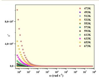
Fig. 8 Frequency dependence of  $\varepsilon'$  at several temperatures.
