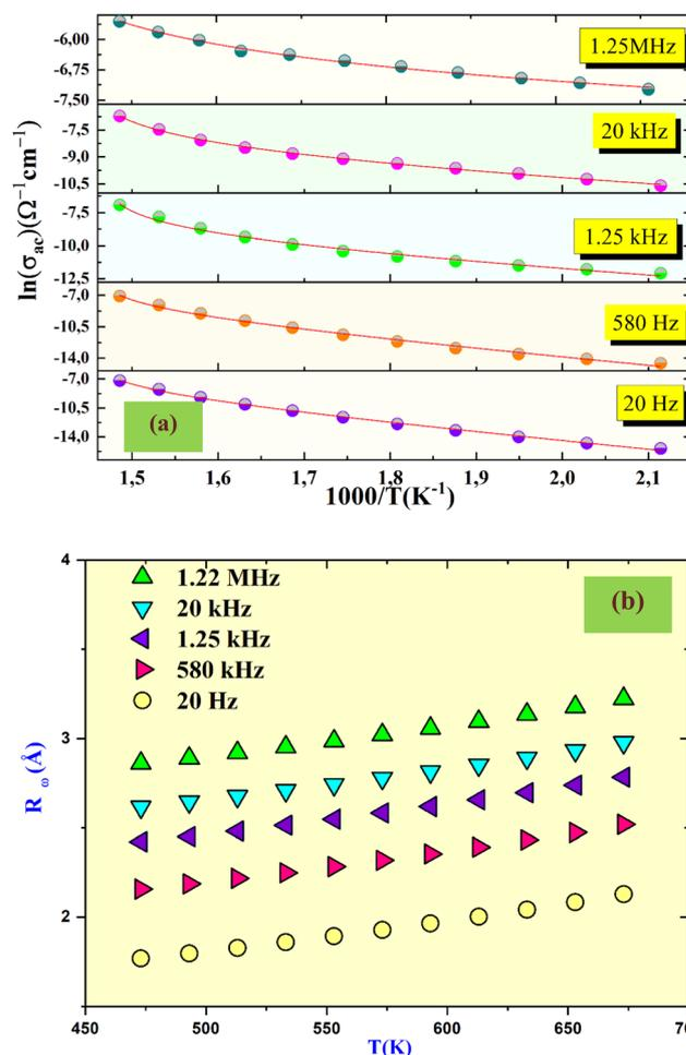
Fig. 4 (a) AC conductivity of  $\text{LiVO}_3$  vs.  $1000/T$  at various frequencies, fitted to the correlated barrier hopping (CBH) model. (b) The temperature dependence of  $R_\omega$  (Å) of  $\text{LiVO}_3$  at different indicated frequencies.
