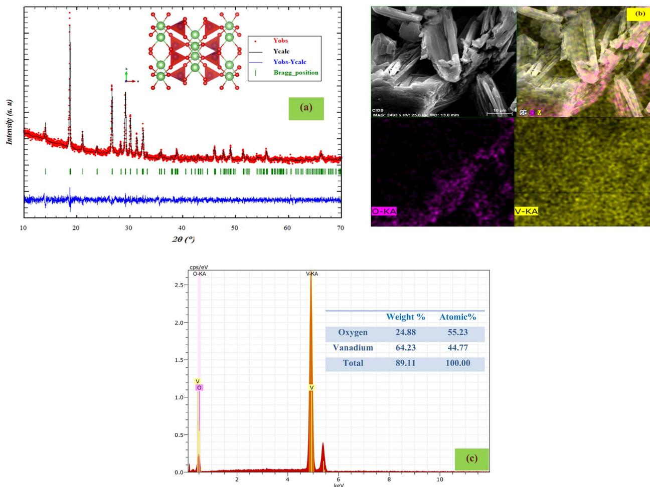
Fig. 1 (a) Powder X-ray diffractogram of  $\text{LiVO}_3$  recorded at room temperature. The inset shows the crystal structure of the  $\text{LiVO}_3$ . (b) Morphological analysis of  $\text{LiVO}_3$  by SEM imaging. (c) Energy-dispersive X-ray (EDX) spectrum and elemental composition analysis.
