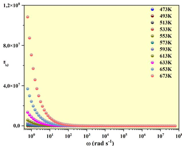
Fig. 9 Frequency dependence of  $\epsilon''$  at several temperatures.
