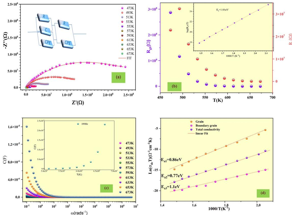
Fig. 2 (a) Nyquist plot with equivalent circuit representation of  $\text{LiVO}_3$ . (b) Temperature dependence of grain ( $R_g$ ) and grain boundary ( $R_{gb}$ ) resistances (inset: plot of  $\ln(R_{gb}/T)$  vs.  $1000/T$ ). (c) Frequency dependence of capacitance at different temperatures. (d) Variation of  $\ln(\sigma_{dc})$  as a function of temperature.
