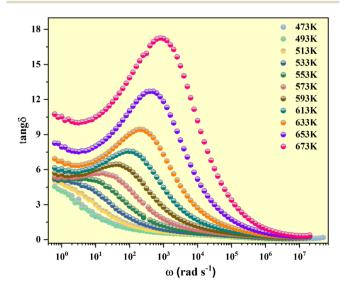
Fig. 10 Frequency dependence of  $tan(\delta)$  at several temperatures.
