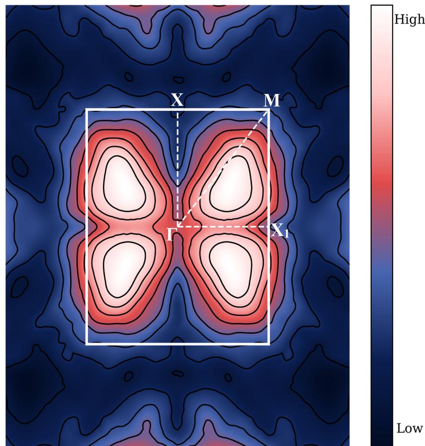
Fig. 7 The Fermi surface nesting function  $\zeta(\vec{Q})$  in the  $k_z = 0$  plane of Nd<sub>3</sub>In. SOC is not considered.
