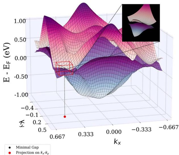
Fig. 9 3D plot of the electronic band structure (with SOC) showing the Weyl point located between the topmost valence and lowest conduction bands. The projection of the Weyl point onto the  $k_x$ - $k_y$  plane is marked with a red dot.
