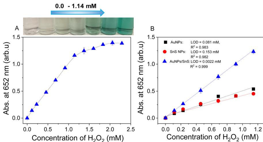
Fig. 6 (A) Calibration curve and (B) linear range for H<sub>2</sub>O<sub>2</sub> detection from 0 to 1.14 mM using AuNPs/SnS nanocomposite ratio of (2 : 1).
