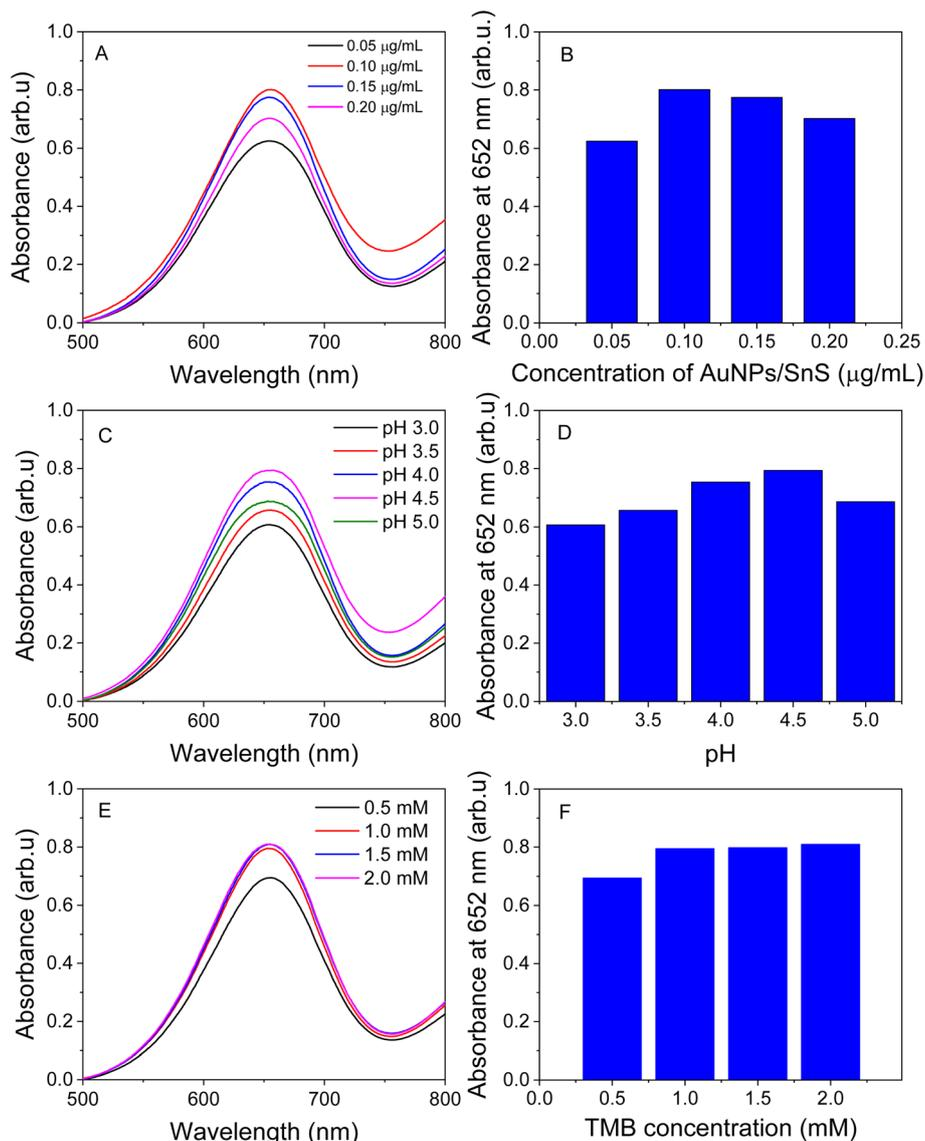
Fig. 5 UV-vis absorption spectra (left) and corresponding absorbance plots at 652 nm (right) for the oxidation of red-TMB using  $\text{H}_2\text{O}_2$  and catalysis of AuNPs/SnS nanocomposite at the (2 : 1) ratio: (A and B) effect of catalyst concentration; (C and D) effect of pH; (E and F) effect of red-TMB concentration.
