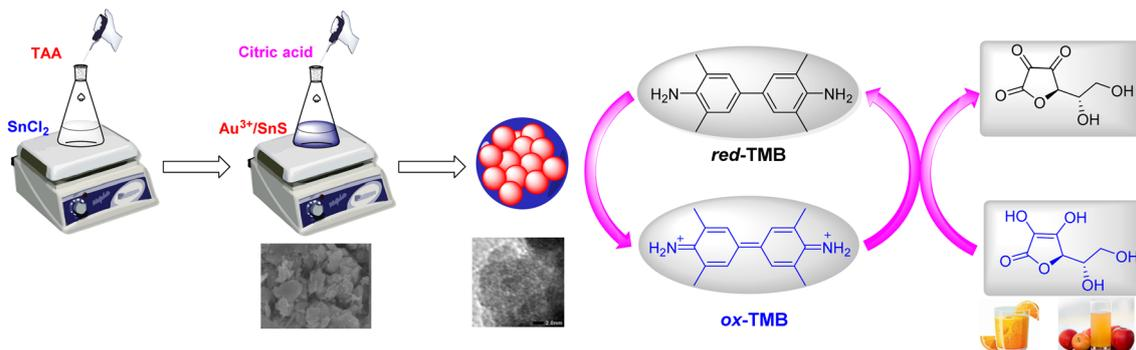
Fig. 1 Schematic illustration of the synthesis of AuNPs/SnS nanoparticles and their peroxidase-mimetic activity for the detection of ascorbic acid.
