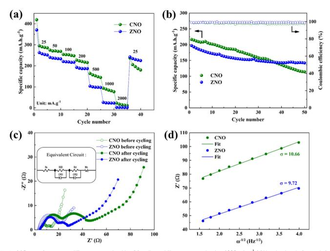
Fig. 5 (a) Rate performance at different current densities, (b) cycling stability at a current density of 200 mA  $g^{-1}$ , (c) Nyquist plots, before and after cycling (inset: equivalent circuit), (d) Z' and  $\omega^{-1/2}$  fitting curves at a low frequency region of CNO and ZNO samples.
