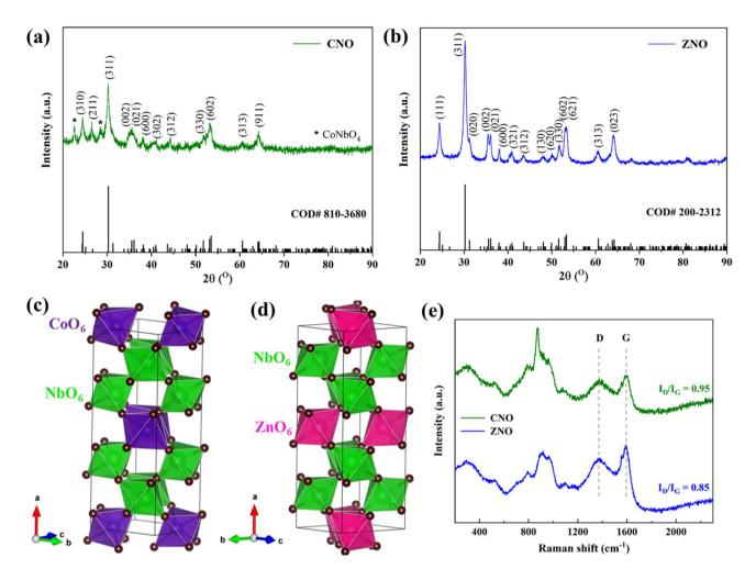
Fig. 1 XRD patterns (a and b), crystal structure (c and d) of CNO and ZNO materials, respectively, and (e) Raman spectra of CNO and ZNO materials.
