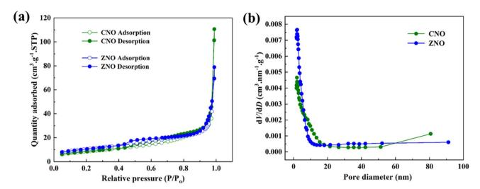
Fig. 3 (a) N<sub>2</sub>-adsorption and desorption isotherms, and (b) pore size distribution of CNO and ZNO materials.
