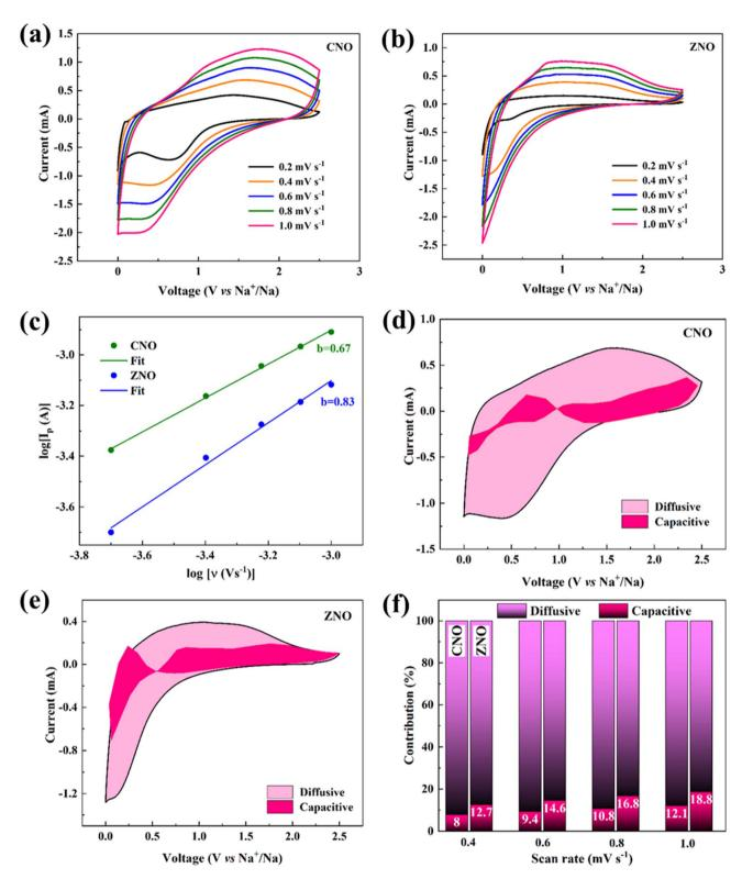
Fig. 6 Cyclic voltammogram at different scan rates for (a) CNO and (b) ZNO materials. (c) Plot of log(v) vs.  $log(i_p)$  of CNO and ZNO materials. CV curve displaying the diffusive and capacitive contribution of (d) CNO, and (e) ZNO materials at 0.4 mV s<sup>-1</sup> scan rate, and (f) percentage contribution of diffusive and capacitive processes at different scan rates for CNO and ZNO samples.
