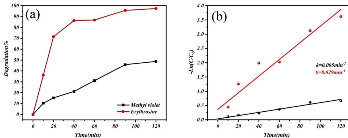
Fig. 7 (a) Photo-degradation of anionic and cationic dyes in the presence of the BF<sub>4</sub> catalyst and (b) the relative plots of first-order degradation.
