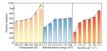
Fig. 11 Statistics of the variation in the number of contaminant particles removed in the plasma cleaning simulation experiment with each experimental parameter.
