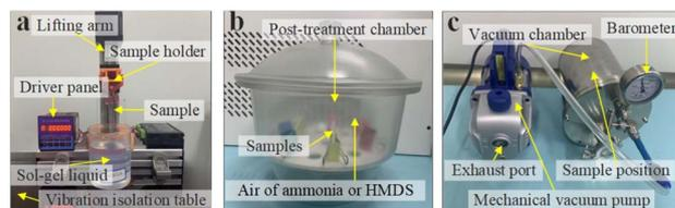
Fig. 1 Experimental sample preparation equipment: (a) lifting coater to deposit chemical coatings on samples; (b) post-treatment of the coating with ammonia and HMDS; and (c) contamination process of the chemical coatings with DBP.
