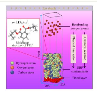
Fig. 5 Molecular dynamics model of the reaction between plasma and organic contaminants.
