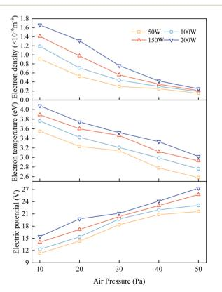
Fig. 7 Single-point Langmuir probe measurement showing the measurement results of electron density, electron temperature and electric potential with different discharge powers and pressures.
