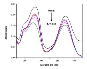
Fig. 12 Photocatalytic detoxification of Cr(IV) to Cr(III) ions in the presence of UV light source (365 nm).
