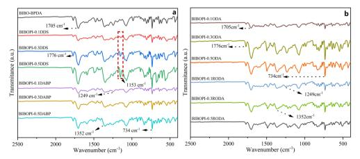
Fig. 2 FTIR spectra of (a) BIBOPIs containing DDS and DABP diamine, (b) BIBOPIs containing ODA and RODA diamine.
