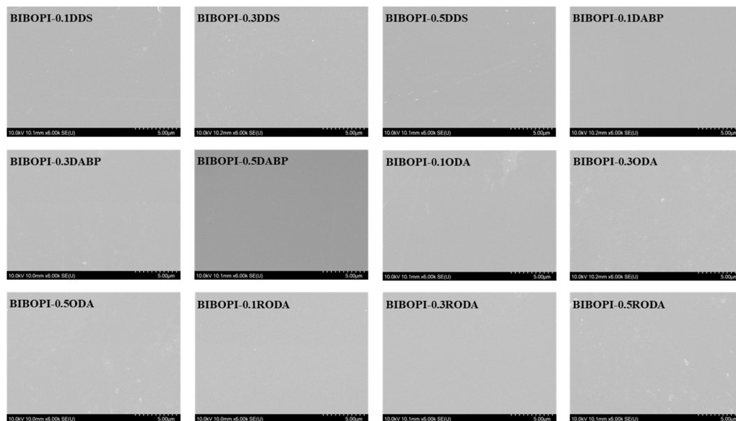
Fig. 7 SEM of BIBOPI coated aluminum substrate.
