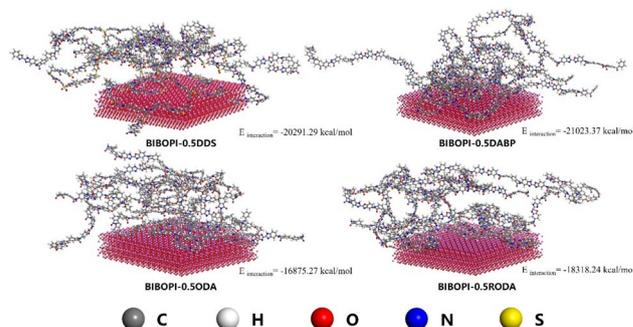
Fig. 6 Simulation of interaction between BIBOPIs and substrates.
