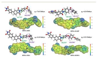
Fig. 1 Optimized geometry and electrostatic potential surfaces of BPDA-DDS, BPDA-DABP, BPDA-ODA and BPDA-RODA polymer structures (color code: H atom, white; C atom, dark gray; N atom, blue; S atom, yellow; O atom, red).
