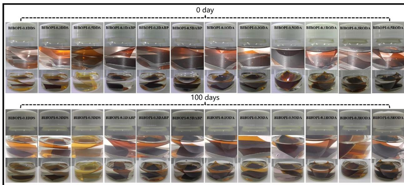
Fig. 4 Electrolyte resistance of BIBOPI films and BIBOPI coated aluminum substrates.
