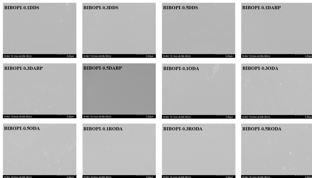
Fig. 7 SEM of BIBOPI coated aluminum substrate.
