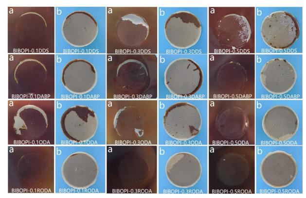
Test results of pull-off experiment (digital photos: (a) film interface; (b) spindle interface)
