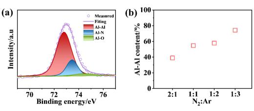
Fig. 3 (a) XPS spectra of the AlN film prepared under  $N_2$ /Ar ratio of 1:3; (b) variation in the Al–Al bond content as determined by fitting the XPS results.
