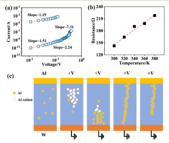
Fig. 4 (a) Logarithmic plots of current (l) versus voltage (V) for the SET and RESET processes and (b) variation of LRS resistance with different temperature prepared at N<sub>2</sub>/Ar ratios of 1:3, (c) schematic illustration of the formation and rupture of conductive filaments in the Al/AlN/W device.
