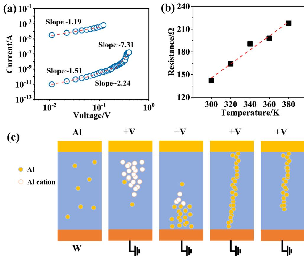
Fig. 4 (a) Logarithmic plots of current ( $I$ ) versus voltage ( $V$ ) for the SET and RESET processes and (b) variation of LRS resistance with different temperature prepared at  $N_2/Ar$  ratios of 1 : 3, (c) schematic illustration of the formation and rupture of conductive filaments in the Al/AlN/W device.
