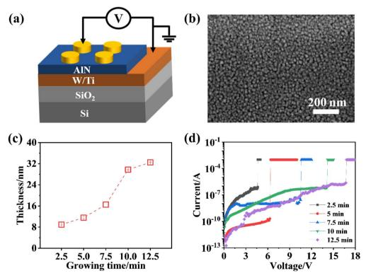
Fig. 1 (a) Schematic diagram of the Al/AlN/W device; (b) surface SEM image; (c) plot of AlN film thickness; (d) I-V electroforming curves of Al/AlN/W devices.
