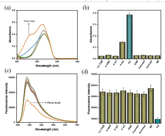
Fig. 2 (a) UV-vis and (c) fluorescence spectra of BMP ( $c=2.0\times10^{-5}$  M) recorded after the addition of various potentially interfering analytes ( $c=2.0\times10^{-4}$  M, 15 equivalents) in CH<sub>3</sub>CN/HEPES buffer (9 : 1, v/v, pH 7.4). Corresponding (b) UV-vis and (d) fluorescence responses of BMP toward the different analytes are presented as bar diagrams (error value, 5%; Y error bar for both [ $\pm$ ] deviation).
