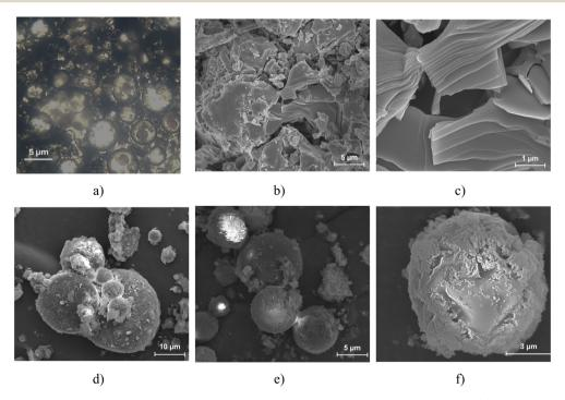
Fig. 2 Morphology characterization of the samples: (a) optical microscopy of the polymer particles; (b) and (c) SEM images of the Mo<sub>2</sub>Ti<sub>2</sub>AlC<sub>3</sub> MAX phase; (d-f) SEM analysis of the poly(MMA-co-HPMA)-MXene polymer microparticles containing MXenes.
