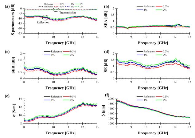
Fig. 9 (a) Measured S parameters. Extracted (b) SE<sub>A</sub>, (c) SE<sub>R</sub>, (d) SE, (e) conductivity, and (f) skin depth for all the MUTs in the X band.
