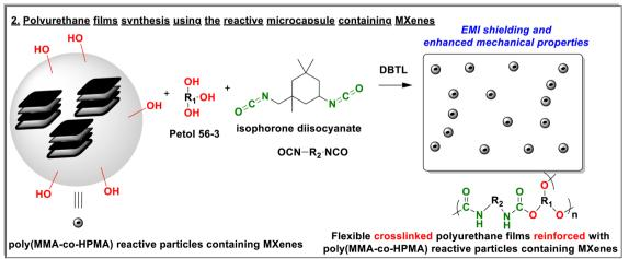
Scheme 1 Concept for using reactive polymer particles containing MXenes as reinforcing agents in polyurethane films and EMI shielding component.
