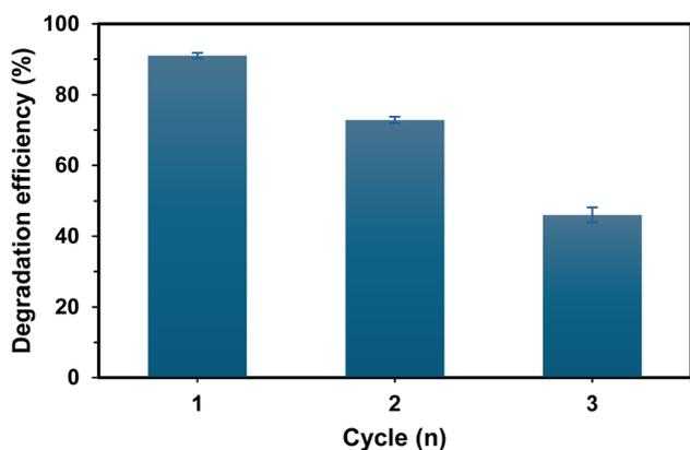
Fig. 14 Reusability of Fe/Ni@ZIF-8 photocatalyst under visible light.
