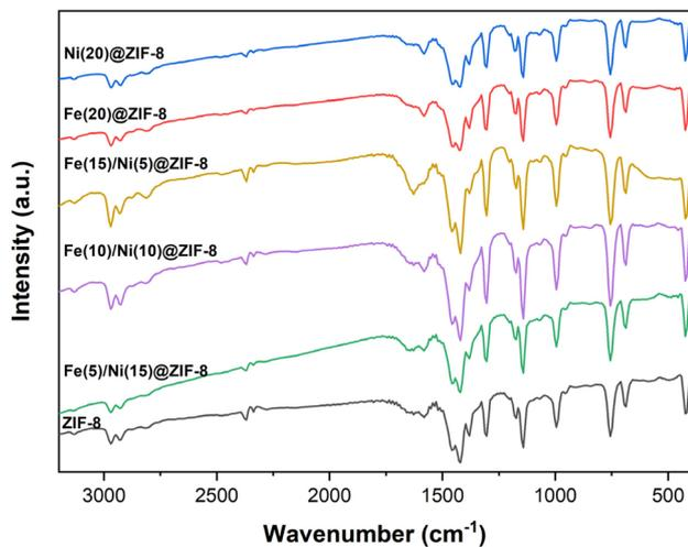
Fig. 2 FTIR spectra of ZIF-8, single doped Fe@ZIF-8 and Ni@ZIF-8, and Fe/Ni@ZIF-8 composites.
