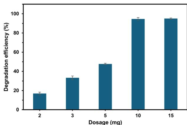
Fig. 11 Photocatalytic activity of Fe(15)/Ni(5)@ZIF-8 at various dosage ( $C_0 = 30$  mg L<sup>-1</sup>,  $V = 10$  mL, pH = 11, vis light = 180 min).
