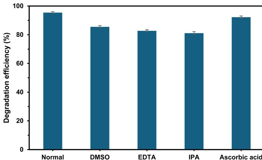
Fig. 13 Trapping experiment ( $W = 10$  mg,  $V = 10$  mL,  $C = 30$  mg L<sup>-1</sup>).
