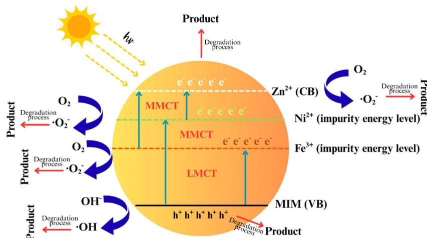
Fig. 15 Proposed diagram of charge migration pathway through LMCT and MMCT on MB degradation mechanism using Fe(15)/Ni(5)@ZIF-8.
