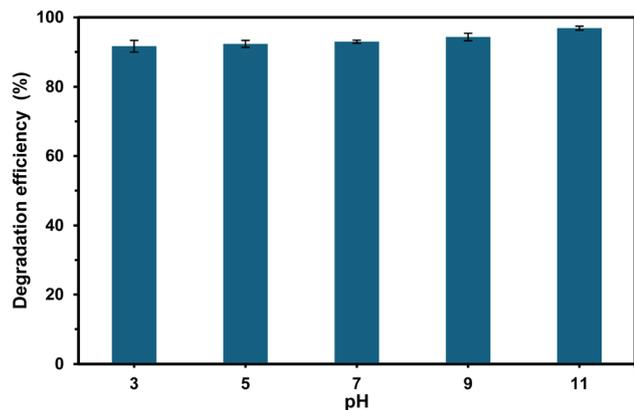
Fig. 10 Photocatalytic activity of Fe(15)/Ni(5)@ZIF-8 at various pH ( $W = 10$  mg,  $V = 10$  mL,  $C = 30$  mg L<sup>-1</sup>, vis light = 180 min).
