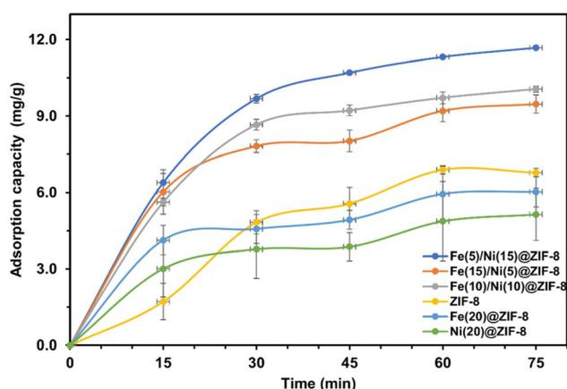
Fig. 8 Adsorption capacity of ZIF-8, Fe@ZIF-8, Ni@ZIF-8, and Fe/Ni@ZIF-8 composites.
