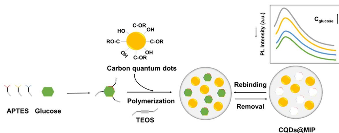
Fig. 7 Schematic illustration of the fabrication process and sensing mechanism of CQDs@MIP.
