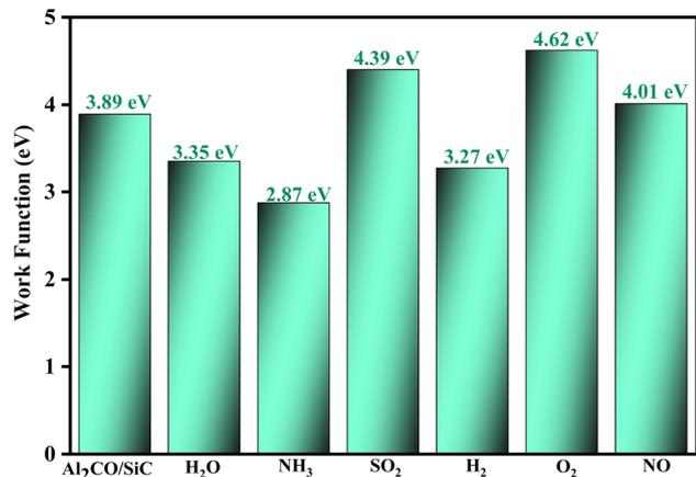
Fig. 7 WF of the Al<sub>2</sub>CO/SiC heterostructure after the adsorption of various gas molecules.
