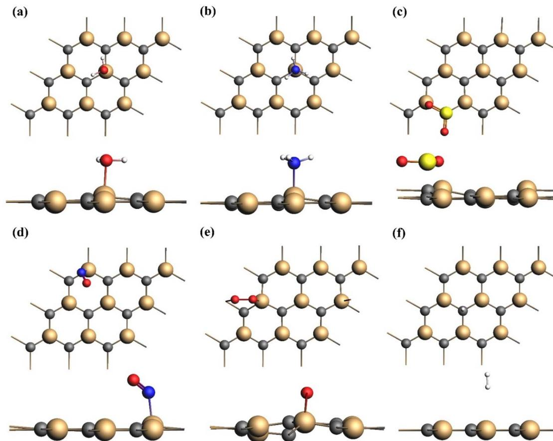
Fig. 3 Top and side views of the most energetically favorable optimized structures of SiC ML with gas adsorption: (a) H<sub>2</sub>O, (b) NH<sub>3</sub>, (c) SO<sub>2</sub>, (d) NO, (e) O<sub>2</sub> and (f) H<sub>2</sub>.
