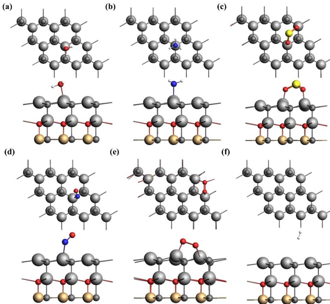
Fig. 6 The most favorable configurations for (a) H<sub>2</sub>O, (b) NH<sub>3</sub>, (c) SO<sub>2</sub>, (d) NO, (e) O<sub>2</sub>, and (f) H<sub>2</sub> adsorbed on the Al<sub>2</sub>CO/SiC heterostructure.
