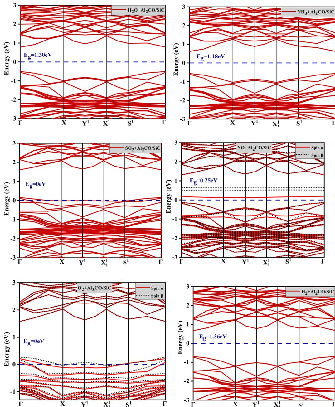
Fig. 8 The calculated band structures of the  $\text{Al}_2\text{CO/SiC}$  heterostructure after the adsorption of different gas molecules  $\text{H}_2\text{O}$ ,  $\text{NH}_3$ ,  $\text{SO}_2$ ,  $\text{NO}$ ,  $\text{O}_2$ , and  $\text{H}_2$ .
