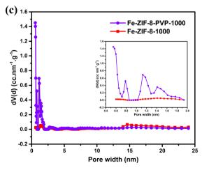
Fig. 5 (a)  $N_2$  adsorption curves of Fe-ZIF-8-PVP-1000 and Fe-ZIF-8-1000; (b) BJH-derived mesoporous size distribution patterns of Fe-ZIF-8-PVP-1000 and Fe-ZIF-8-1000; (c) DFT pore size distribution of Fe-ZIF-8-1000 and Fe-ZIF-8-PVP-1000 with emphasis on micropore region.
