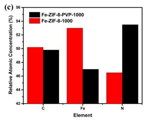
Fig. 3 (a) XRD patterns of Fe-ZIF-8-PVP-1000 and Fe-ZIF-8-1000, (b) XPS survey spectrum of Fe-ZIF-8-PVP-1000 and Fe-ZIF-8-1000, and (c) relative atomic distribution (by XPS) in Fe-ZIF-8-1000 and Fe-ZIF-8-PVP-1000.
