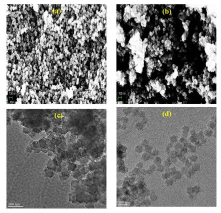
Fig. 1 SEM images of (a) Fe-ZIF-8-PVP-1000 and (b) Fe-ZIF-8-1000, and TEM images of (c) Fe-ZIF-8-PVP-1000 and (d) Fe-ZIF-8-1000.
