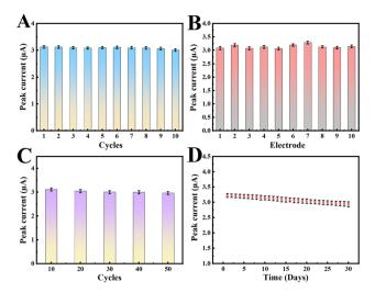
Repeatability evaluation of the CS/UiO-66-NH<sub>2</sub>/SA-2-based electroanalytical sensor (A); analysis of the reproducibility of CS/UiO-66-NH<sub>2</sub>/SA-2/GCE with 10 independent electrodes (B); cyclic stability (C) and storage stability (D) of CS/UiO-66-NH $_2$ /SA-2/GCE (0.1 mol L $^-$ PBS, pH = 6.0).
