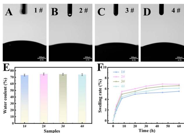
Fig. 2 Contact angles (A)–(D), water contents (E) and swelling rates (F) of CS/SA (1#), CS/UiO-66-NH<sub>2</sub>/SA-1 (2#), CS/UiO-66-NH<sub>2</sub>/SA-2 (3#) and CS/UiO-66-NH<sub>2</sub>/SA-3 (4#).
