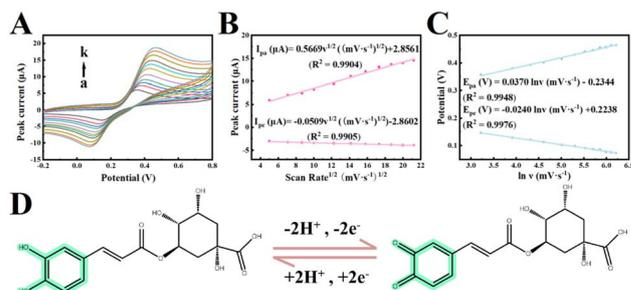
Fig. 7 CV profiles of CS/UiO-66-NH<sub>2</sub>/SA-2/GCE for 100 μmol L<sup>-1</sup> CGA at different scan rates (a–k: 25–450 mV s<sup>-1</sup>) (0.1 mol L<sup>-1</sup> PBS, pH = 6.0) (A); linear relationship of oxidation/reduction peak current vs.  $\nu^{1/2}$  (B); functional relationship between redox potential and  $\ln \nu$  (C); and electroanalytical reaction equation of CGA (D).
