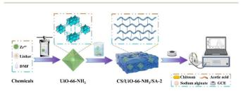
Scheme 1 Schematic of the synthesis route of CS/UiO-66-NH<sub>2</sub>/SA-2.
