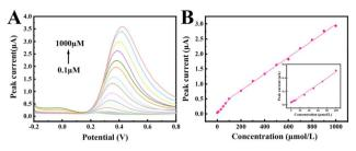
Fig. 8 DPV signals of CGA on CS/UiO-66-NH<sub>2</sub>/SA-2/GCE in  $0.1 \text{ mol L}^{-1} \text{ PBS (pH} = 6.0)$  (A) and linear plot of current versus CGA concentration (B); inset: linear curve at low concentrations (0.1-100  $\mu$ mol L<sup>-1</sup>)
