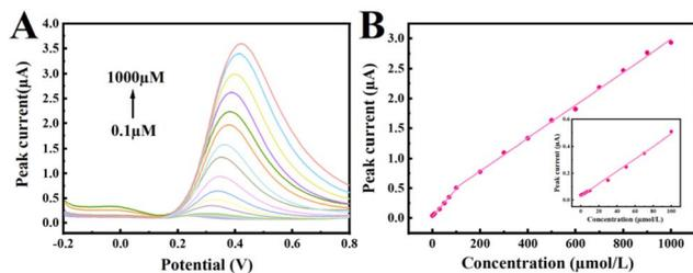
Fig. 8 DPV signals of CGA on CS/UiO-66-NH<sub>2</sub>/SA-2/GCE in 0.1 mol L<sup>-1</sup> PBS (pH = 6.0) (A) and linear plot of current versus CGA concentration (B); inset: linear curve at low concentrations (0.1–100 μmol L<sup>-1</sup>).
