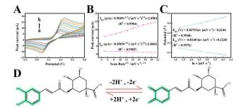
Fig. 7 CV profiles of CS/UiO-66-NH<sub>2</sub>/SA-2/GCE for 100  $\mu$ mol L<sup>-1</sup> CGA at different scan rates (a–k: 25–450 mV s<sup>-1</sup>) (0.1 mol L<sup>-1</sup> PBS, pH = 6.0) (A); linear relationship of oxidation/reduction peak current vs.  $v^{1/2}$  (B); functional relationship between redox potential and ln v (C); and electroanalytical reaction equation of CGA (D).
