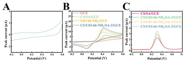
Fig. 5 CV curves of CS/UiO-66-NH<sub>2</sub>/SA-2/GCE in PBS solution without CGA (A) and CV curves (B) and DPV curves (C) for a series of modified electrodes in PBS solution containing CGA (pH = 6.0).
