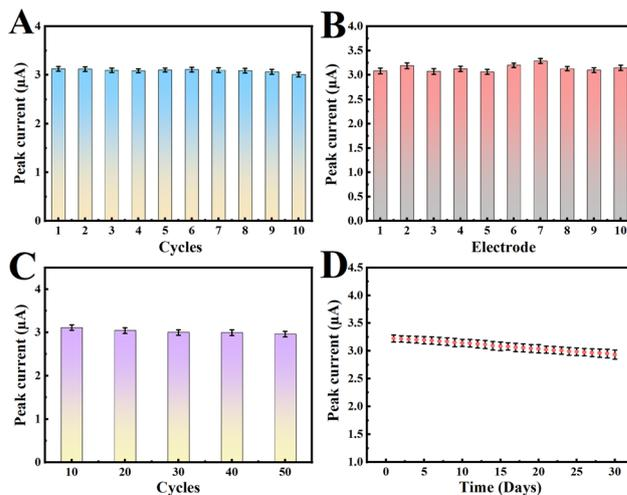
Fig. 9 Repeatability evaluation of the CS/UiO-66-NH<sub>2</sub>/SA-2-based electroanalytical sensor (A); analysis of the reproducibility of CS/UiO-66-NH<sub>2</sub>/SA-2/GCE with 10 independent electrodes (B); cyclic stability (C) and storage stability (D) of CS/UiO-66-NH<sub>2</sub>/SA-2/GCE (0.1 mol L<sup>-1</sup> PBS, pH = 6.0).
