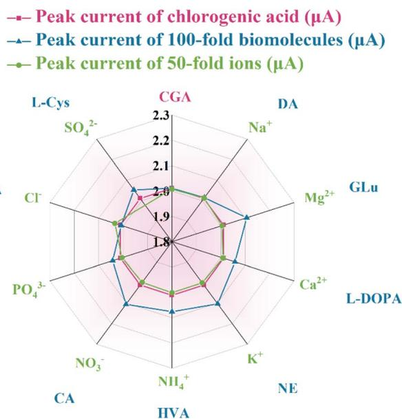
Fig. 10 Radar plot showing the impact of different types of interferences on the CGA response in 0.1 mol L<sup>-1</sup> PBS (pH = 6.0) using CS/Uio-66-NH<sub>2</sub>/SA-2/CGE.
