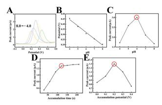
Fig. 6 DPV curves of CS/UiO-66-NH<sub>2</sub>/SA-2/GCE in 0.1 mol L<sup>-1</sup> PBS (pH = 4.0–8.0) solution containing 100  $\mu$ mol L<sup>-1</sup> CGA (A); relationship between pH value and potential (B); peak current at different pH values (C); and influence of enrichment time (D) and enrichment potential (E) on peak current of CGA (0.1 mol L<sup>-1</sup> PBS, pH = 6.0).
