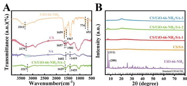
Fig. 3 FT-IR spectra of UiO-66-NH<sub>2</sub>, CS, SA and CS/UiO-66-NH<sub>2</sub>/SA-2 (A) and XRD profiles of UiO-66-NH<sub>2</sub>, CS/SA, CS/UiO-66-NH<sub>2</sub>/SA-1, CS/UiO-66-NH<sub>2</sub>/SA-2 and CS/UiO-66-NH<sub>2</sub>/SA-3 (B).
