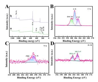
Fig. 4 XPS broad spectrum (A) of UiO-66-NH<sub>2</sub> (a) and CS/UiO-66-NH<sub>2</sub>/SA-2 (b) and C 1s (B), N 1s (C), and Zr 3d (D) spectra of CS/UiO-66-NH2/SA-2.
