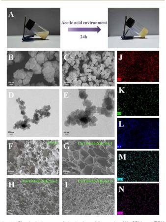
Fig. 1 Physical diagram of the hydrogel formation (A); SEM and TEM images of UiO-66-NH<sub>2</sub> at different magnifications (B)-(E); SEM images of CS/SA, CS/UiO-66-NH<sub>2</sub>/SA-1, CS/UiO-66-NH<sub>2</sub>/SA-2, and CS/UiO-66-NH<sub>2</sub>/SA-3 (F)-(I); and elemental mapping of CS/UiO-66-NH<sub>2</sub>/SA-2(J)-(N)
