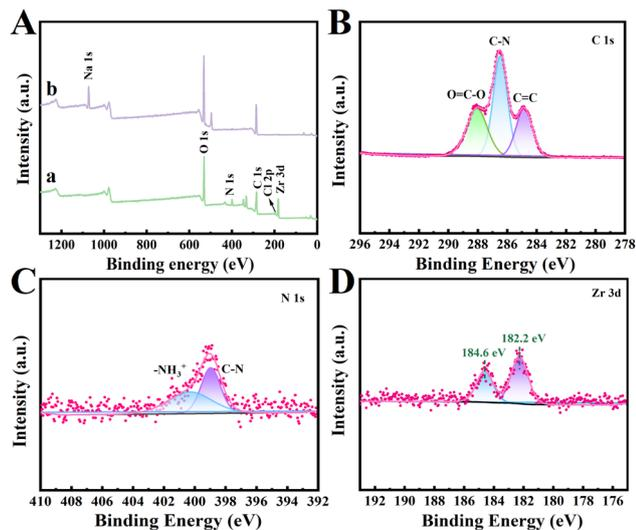
Fig. 4 XPS broad spectrum (A) of UiO-66-NH<sub>2</sub> (a) and CS/UiO-66-NH<sub>2</sub>/SA-2 (b) and C 1s (B), N 1s (C), and Zr 3d (D) spectra of CS/UiO-66-NH<sub>2</sub>/SA-2.
