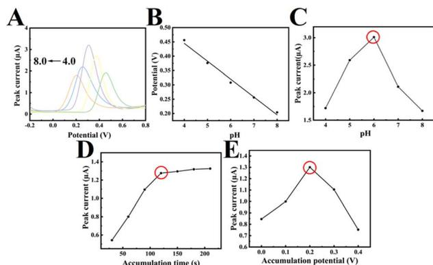
Fig. 6 DPV curves of CS/UiO-66-NH<sub>2</sub>/SA-2/GCE in 0.1 mol L<sup>-1</sup> PBS (pH = 4.0–8.0) solution containing 100 μmol L<sup>-1</sup> CGA (A); relationship between pH value and potential (B); peak current at different pH values (C); and influence of enrichment time (D) and enrichment potential (E) on peak current of CGA (0.1 mol L<sup>-1</sup> PBS, pH = 6.0).
