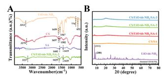
Fig. 3 FT-IR spectra of UiO-66-NH $_2$ , CS, SA and CS/UiO-66-NH $_2$ /SA-2 (A) and XRD profiles of UiO-66-NH $_2$ , CS/SA, CS/UiO-66-NH $_2$ /SA-1, CS/UiO-66-NH $_2$ /SA-2 and CS/UiO-66-NH $_2$ /SA-3 (B).
