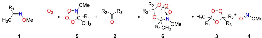
Fig. 2 Mechanism of the Griesbaum co-ozonolysis reaction.
