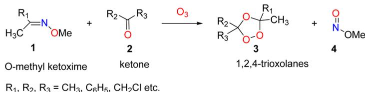
Fig. 1 General scheme of the Griesbaum co-ozonolysis reaction.
