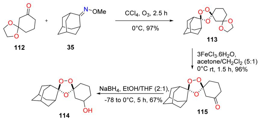
Fig. 22 Synthesis of the 3-keto trioxolane alcohol derivative.
