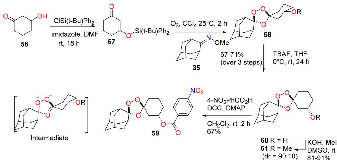
Fig. 13 Stereocontrolled synthesis of the 3-substituted cyclohexane derivative.
