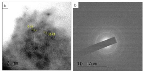
Fig. 8 (a) TEM image and (b) SAED pattern of CONP-NaBH<sub>4</sub>.
