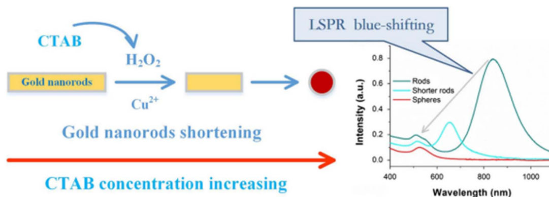
Fig. 9 Shape changes leading to LSPR blue shift of gold nanorods etched by Cu 2+ -mediated H 2 O 2 oxidation in the presence of CTAB. This figure has been adapted from ref. 267 with permission from Springer, copyright 2014.
