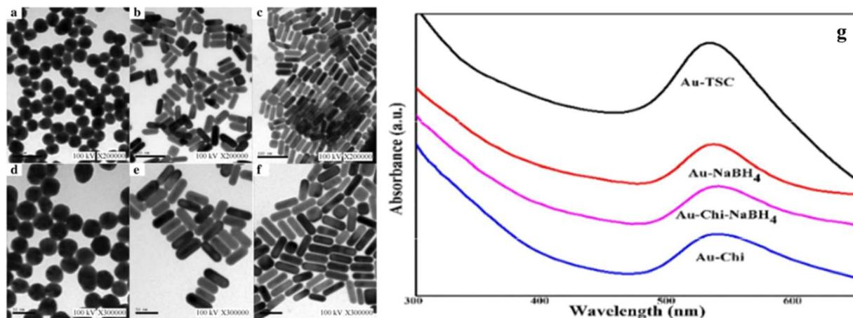
Fig. 4 TEM images of gold nanoparticles with different shapes. (a and d) Spherical nanoparticles, (b and e) short nanorods (c and f) long nanorods<sup>187</sup> (g) the UV-vis spectroscopy of synthesized AuNPs (size range <20 nm) by using different reducing agents. This figure has been adapted from ref. 140 with permission from Royal Society of Chemistry, copyright 2016.
