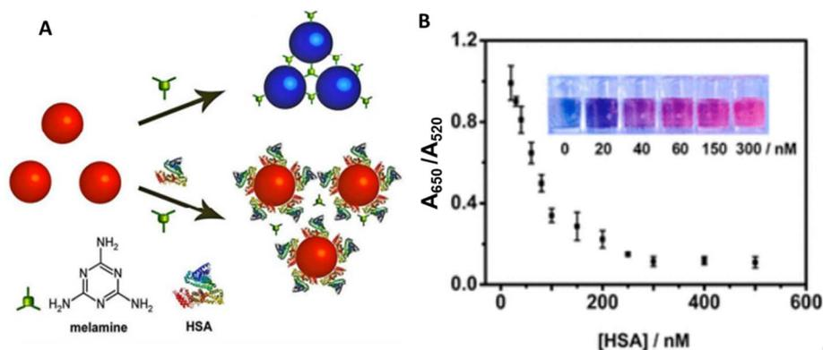
Fig. 15 (A) Schematic illustration of the anti-aggregation effect induced by HSA. (B) Optical photographs of the AuNPs with different conc. of HSA and graph  $A_{650}/A_{520}$  vs. [HSA]/nM. This figure has been adapted from ref. 429 with permission from American Chemical Society, copyright 2015.
