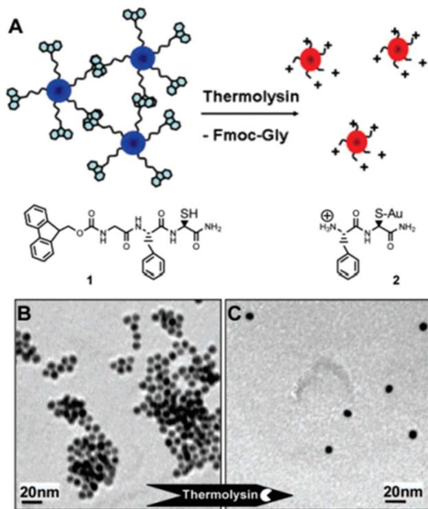
Fig. 16 (A) Schematic representation of the thermolysin-triggered AuNP dispersion approach. (B) TEM image of peptide-AuNPs 1 (8.5 nm at pH 8) (C) TEM image after the addition of thermolysin and formed 2. This figure has been adapted from ref. 431 with permission from PNAS, copyright 2006.
