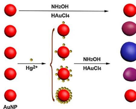
Fig. 7 The schematic illustration of the amount of  $\text{Hg}^{2+}$  on the surface which controls the growth of AuNPs. Reproduced with permission from reference. This figure has been adapted from ref. 236 with permission from Elsevier, copyright 2017.
