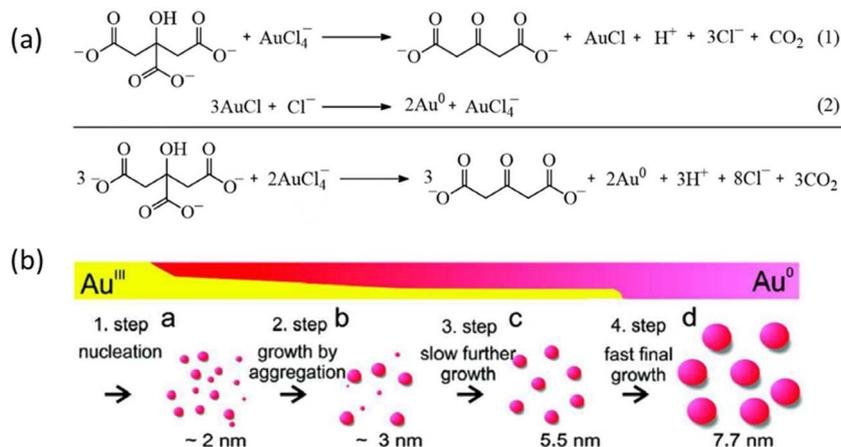
Fig. 1 (a) Accepted reduction mechanism of  $AuCl_4^-$  using citrate in two step redox reaction. (b) Synthesis of spherical AuNPs in the size range of 10–20 nm by Turkevich method.<sup>46</sup> This figure has been adapted from ref. 46 with permission from American Chemical Society, copyright 2010.
