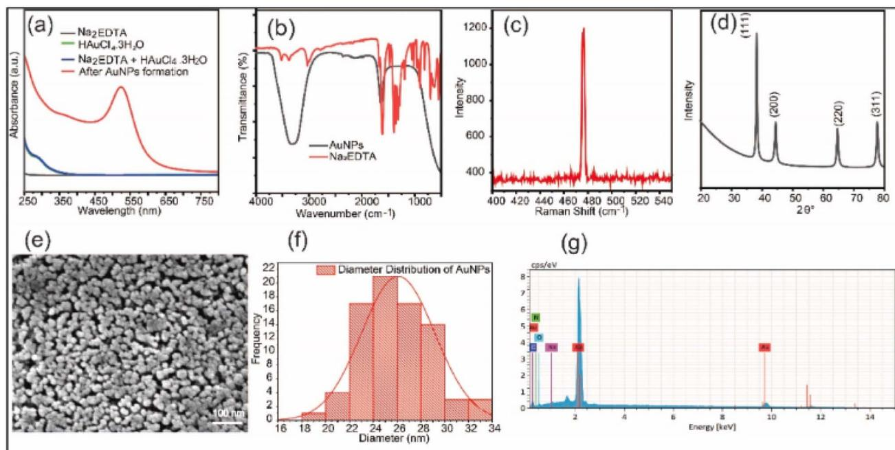
Fig. 5 (a) UV-visible spectrum of the formation of AuNPs. (b) IR spectrum of Na<sub>2</sub>EDTA and synthesized AuNPs solution. (c) Raman spectrum of AuNPs. (d) XRD spectrum of synthesized AuNPs solution. (e) Morphological analysis of the synthesized AuNPs using SEM. (f) Diameter distribution of AuNPs using ImageJ software. (g) EDX spectra analysis of the AuNPs. This figure has been adapted from ref. 167 with permission from Elsevier, copyright 2025.
