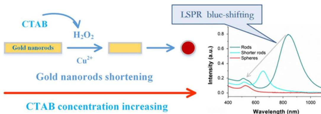
Fig. 9 Shape changes leading to LSPR blue shift of gold nanorods etched by Cu<sup>2+</sup>-mediated H<sub>2</sub>O<sub>2</sub> oxidation in the presence of CTAB. This figure has been adapted from ref. 267 with permission from Springer, copyright 2014.
