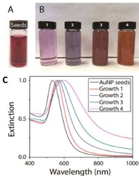
Fig. 3 Seed-mediated growth of varying sizes of spherical gold nanoparticles. (A)  $\sim 40$  nm Au nanoparticles act as seeds in the seed-mediated synthesis. (B) Images of nanoparticle growth after seed-mediated synthesis of group 1, group 2, group 3, and group 4. (C) The extinction spectra of groupwise synthesized AuNP seeds. This figure has been adapted from ref. 61 with permission from American Chemical Society, copyright 2024.
