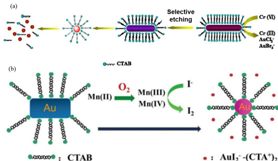
Fig. 10 (a) Schematic illustration on the etching mechanism of the AuNRs induced by Cr(vi). Reproduced with the permission.<sup>279</sup> (b) The schematic illustration for the detection of dissolved oxygen based on the iodine-mediated etching of AuNRs. This figure has been adapted from ref. 265 with permission from Royal Society of Chemistry, copyright 2016.
