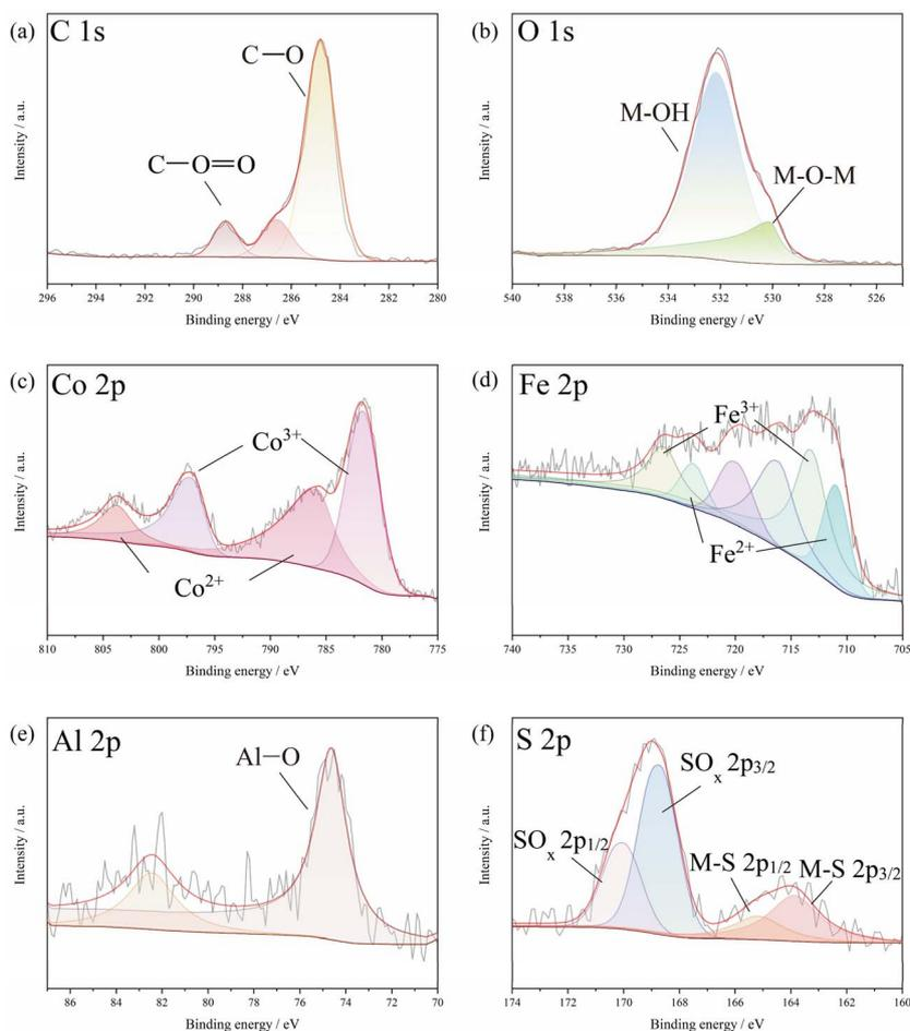
Fig. 4 XPS spectra of C 1s (a), O 1s (b), Co 2p (c), Fe 2p (d), Al 2p (e), and S 2p (f) of S/CoFeAl-LDH.
