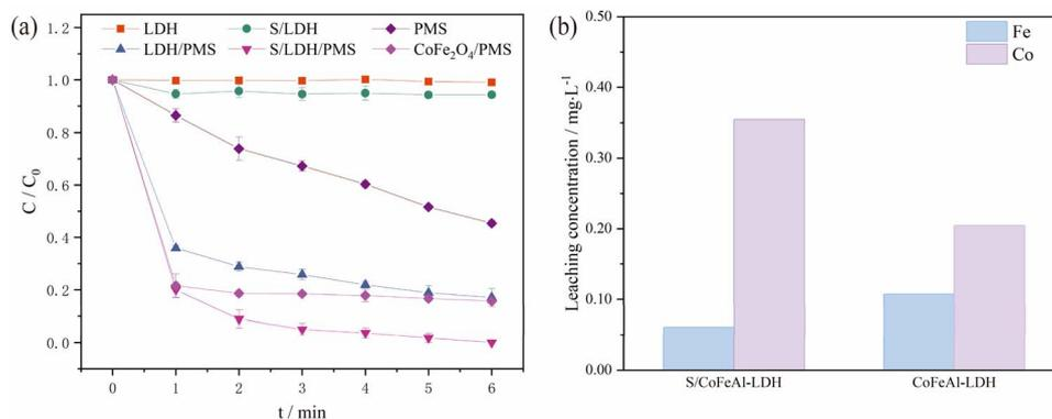
Fig. 5 Removal of NOR under different systems (a) and leaching concentration of cobalt and iron after degradation (b). Reaction conditions:  $C_{\text{catalyst}} = 0.1 \text{ g L}^{-1}$ ,  $C_{\text{PMS}} = 0.2 \text{ g L}^{-1}$ ,  $C_{\text{NOR}} = 20 \text{ mg L}^{-1}$ , initial pH = 6.8.
