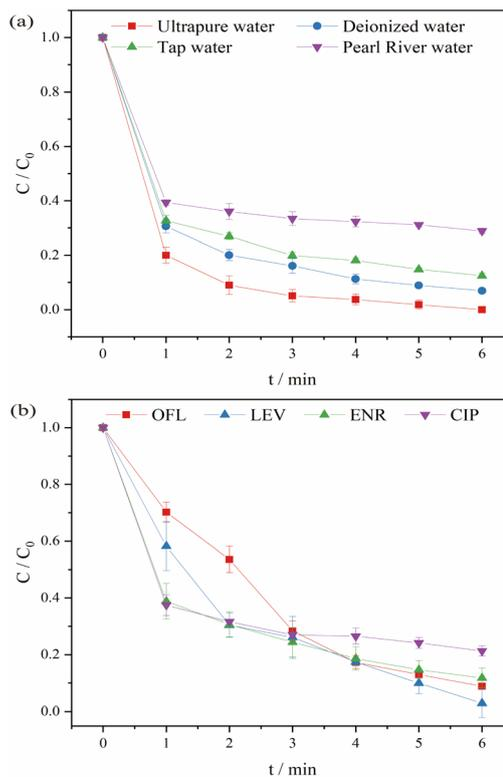
Fig. 7 Removal of NOR in different water samples (a) and Removal of different antibiotics (b) by the S/CoFeAl-LDH/PMS system. Reaction conditions:  $c_{\text{catalyst}} = 0.1 \text{ g L}^{-1}$ ,  $c_{\text{PMS}} = 0.2 \text{ g L}^{-1}$ , initial pH = 6.8,  $c_{\text{NOR}} = c_{\text{OFL}} = c_{\text{LEV}} = c_{\text{ENR}} = c_{\text{CIP}} = 20 \text{ mg L}^{-1}$ .
