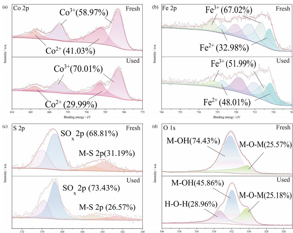
Fig. 9 XPS patterns of the fresh and the used S/CoFeAl-LDH: Co 2p (a), Fe 2p (b), S 2p (c) and O 1s (d).
