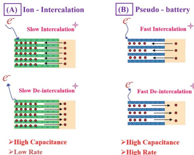
Fig. 5 Schematic view of different charge storage mechanisms (A) charge storage mechanism of rechargeable battery that is ion-intercalation; (B) charge storage mechanism of fast intercalation pseudo-battery.<sup>21</sup> [Reproduced from ref. 21 with permission from The Royal Society of Chemistry, copyright 2025].
